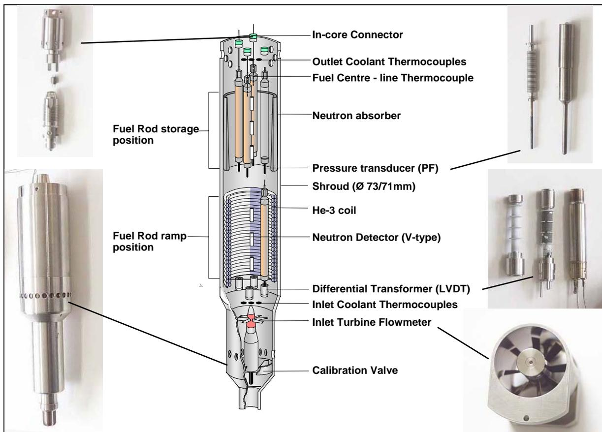
FIG. 2. Example of instrumentation available for a fuel power ramp test assembly in the Halden Reactor.
