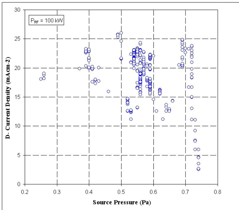
Figure 2: The effect source filling pressure for 100 kW RF power is shown for the total data set for all deuterium shots made on BATMAN since January 2005.
