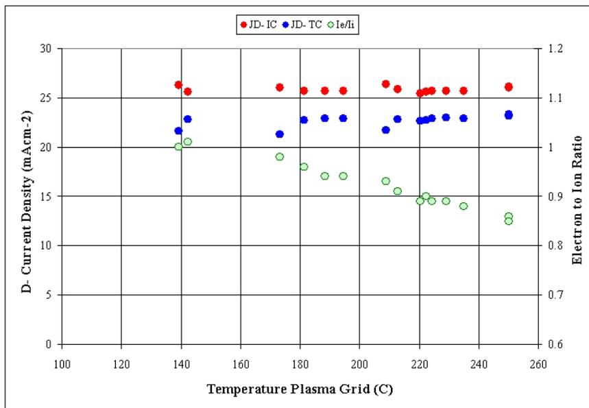
Figure 4: Shown in this figure is the variation of calorimetric (blue) and electrical (red) ion current density plus the electron to ion ratio (green) with plasma grid temperature.
