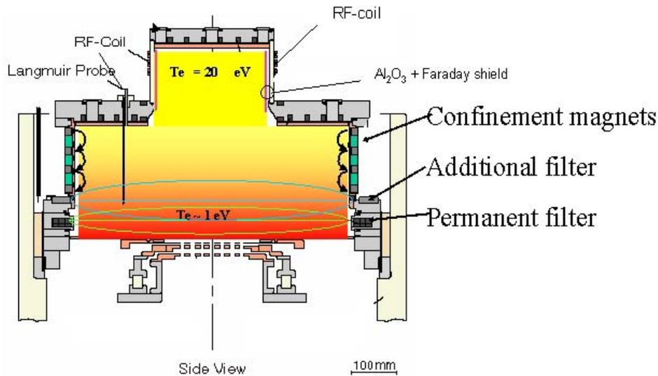
*Figure 6: Shown here is the additional magnet bars and wall confinement magnets added to the normal source configuration to test the effect of different magnetic configurations on source performance.*
