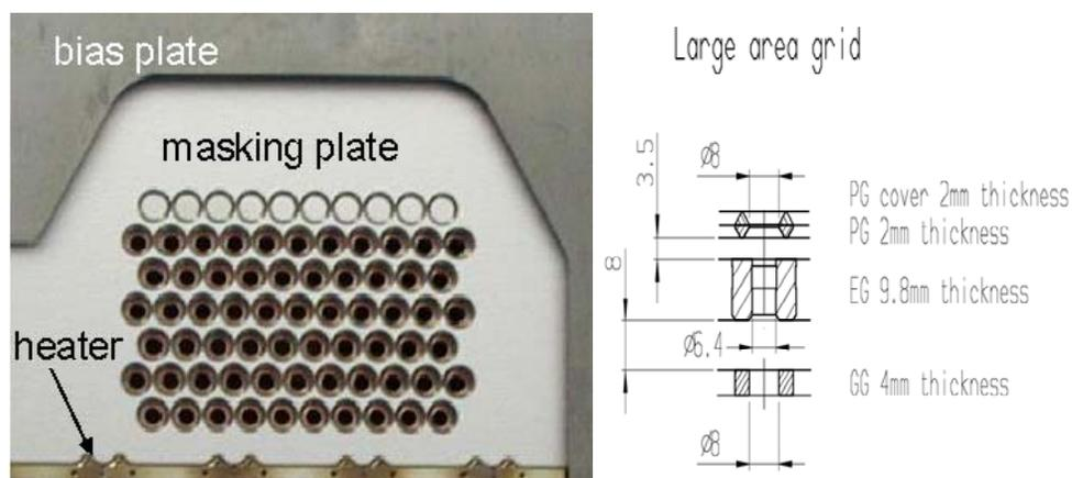
Figure 5: Shown is a picture of the new LAG configuration with the row of holes near the heating element blocked off and the chamfered plate attached. Next to this is a drawing giving details of the extraction geometry.
