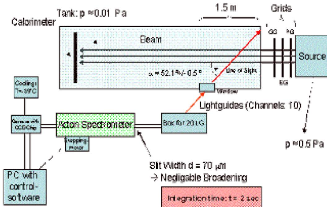
Figure 9: A schematic of the H $\alpha$  emission spectroscopy experimental arrangement on BATMAN.
