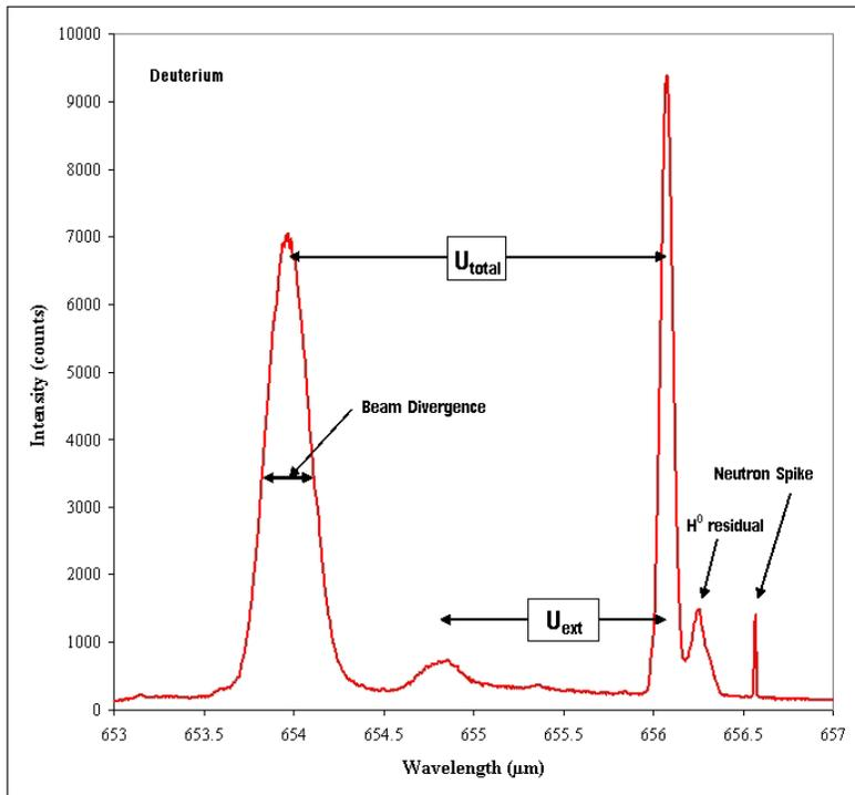
Figure 10: A typical  $H\alpha$  spectrum for deuterium is shown above.
