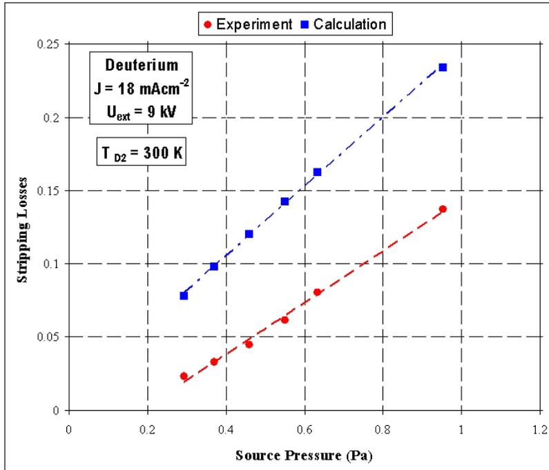
Figure 11: The effect of source pressure on both the measured and theoretical stripping losses for BATMAN are shown. The difference between the theoretical and measured values is due to the assumption of 300 K for the temperature of the gas in constant temperature of  $T = 300\text{ K}$  has been assumed. The potential  $U(x)$  can be measured at each grid.
