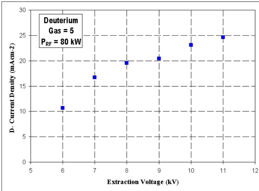
Figure 3: For deuterium shots at gas setting 5, and RF power 80 kW shown above is the effect on calorimetrically measured ion current of variations in the extraction voltage.
