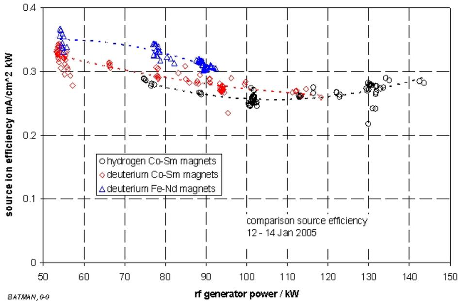
Figure 8: A comparison of source efficiency for hydrogen and deuterium with identical magnetic configuration, plus it also shows the effect of stronger wall confinement magnets for deuterium.
