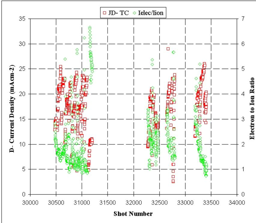
Figure 1: The current density and ion to electron ratio are shown above for the total data set for all deuterium shots made on BATMAN since January 2005.
