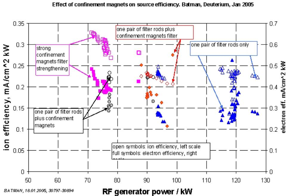
Figure 7: Shown is the effect on source efficiency of different magnetic configurations.
