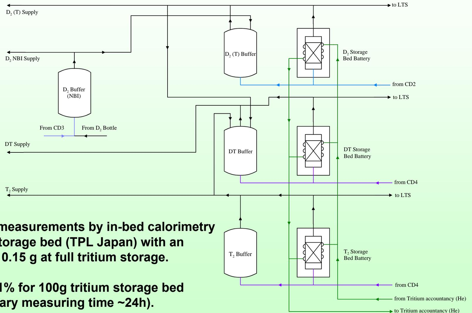
**Tritium inventory measurements by in-bed calorimetry on a 25 g tritium storage bed (TPL Japan) with an accuracy of about 0.15 g at full tritium storage.**
