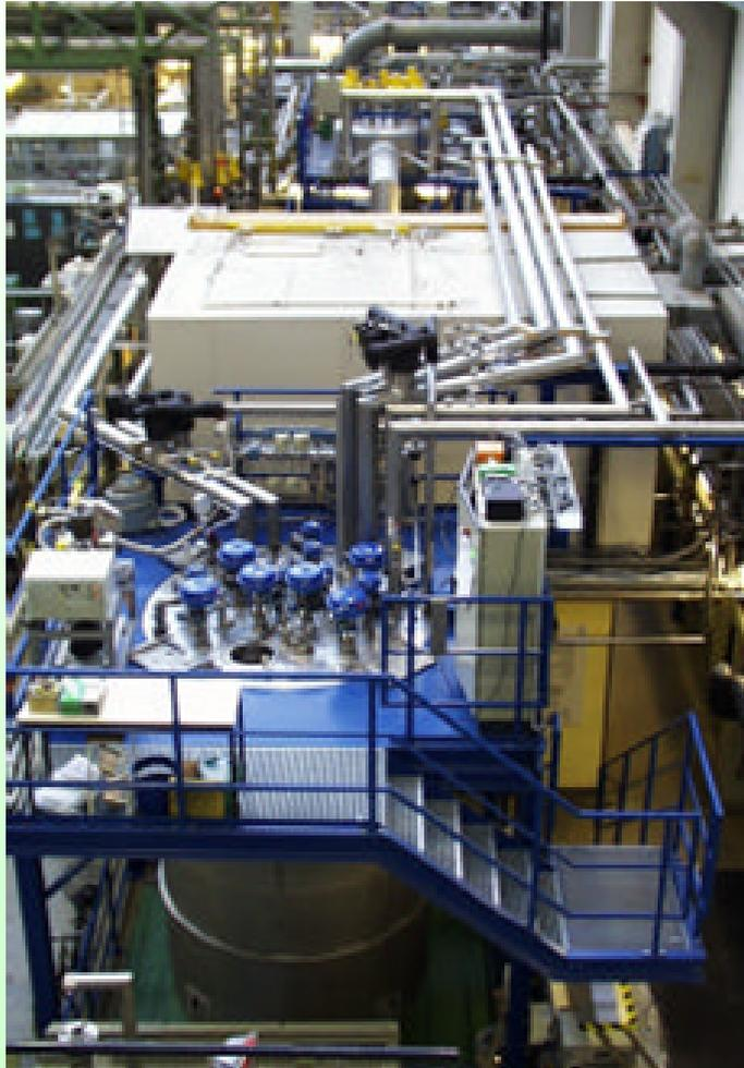
The cryopump is a 1:2 scale model (pumping speed of 50 m<sup>3</sup>/s for DT) of the ITER 1998
