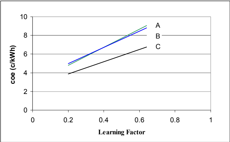
Figure 10: The cost of electricity reduces as technological learning reduces the learning factor. A tenth of a kind plant would be expected to lie around a learning factor of 0.5, whilst a 100 th of a kind plant would be around 0.3. The learning factor is only applied to the fusion specific cost items.
