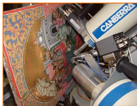
Fig. 2. Schematic drawing of the external ion-beam set-up (left). The photo at right shows the analysis of a painting from the Valadoros Collection, 18th cent., belonging to the Benaki Museum, Athens, Greece.
