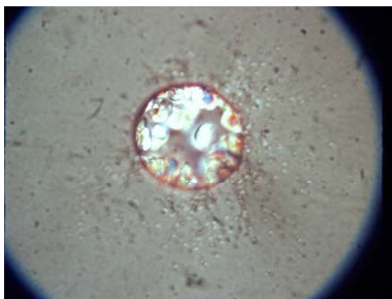
Fig. 3: Left: pico-droplet (Co 1g/L) printed by a modified HP500C on a silicon wafer investigated with a light microscope. Right: Five times 1 droplet of a 1g/L Co standard solution was printed successively with HP 500C on a quartz reflector
