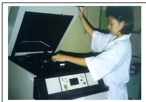
Fig. 1. The PNRI Kevex 771 secondary target XRF spectrometer. On right are air filters mounted on EPA-type filter holders.
