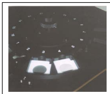
Fig. 1. The PNRI Kevex 771 secondary target XRF spectrometer. On right are air filters mounted on EPA-type filter holders.
