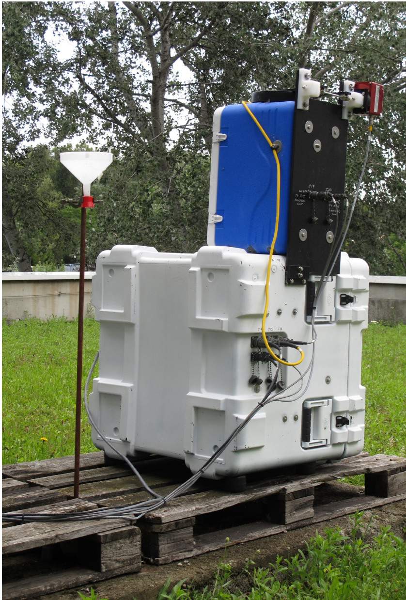
Automated precipitation sampler at the IAEA Isotope Hydrology Laboratory. The sampler was designed and manufactured by T. Coplen (USGS) (photo credit: IAEA).
