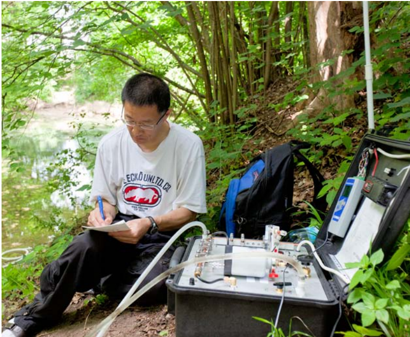
The IHL has been developing a gas sampling device that enables the time-efficient sampling of dissolved gas in water in a smaller package that can be carried to the field like a suitcase (photo credit: IAEA).
