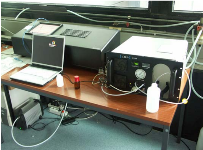
Laser spectroscopy analyzer for water vapour isotope analysis for continuous water vapour isotopes measurement in surface water vapour (photo credit: IAEA).
