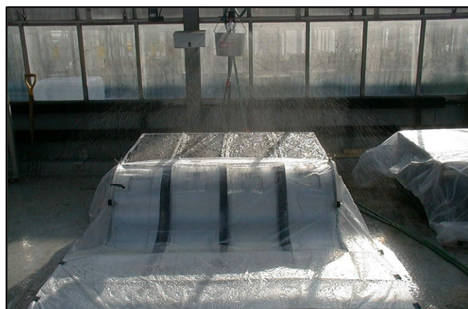
Fig. 4 Rainfall simulation on experimental soil equipped plots (Courtesy of L. Mabit and C. Bernard)
