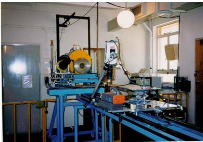
FIG. 2. Calibration set-up for a linearity check of a contamination monitor in front of a multiple source head.
