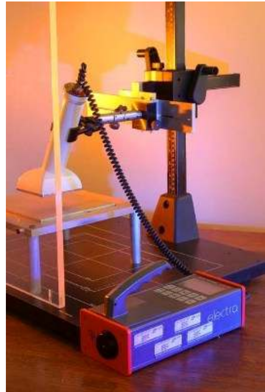
FIG. 3. Calibration set-up of a contamination monitor for 2\pi efficiency and surface activity response.
