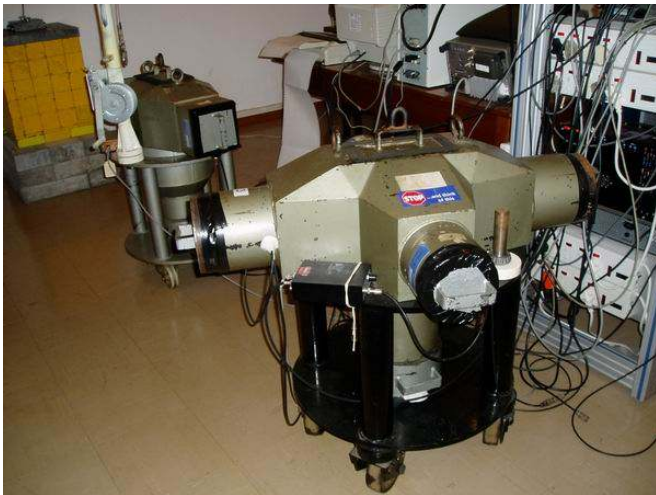
FIG. 5. Liquid scintillation counting system that houses three phototubes and a NaI(Tl) detector. The apparatus forms the basis of a number of absolute counting techniques.
