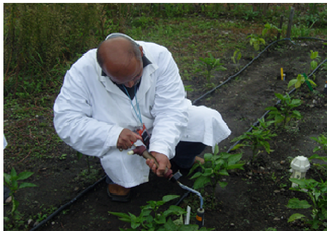
Research fellow sampling soil water using suction cup samplers
