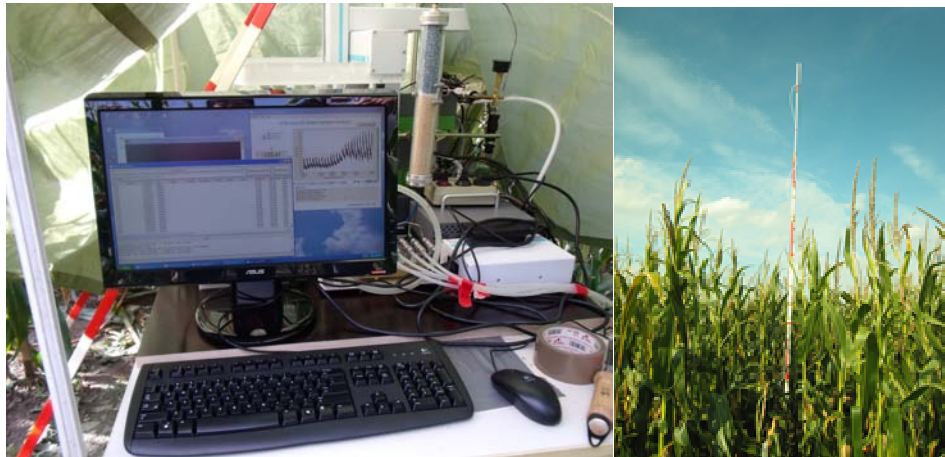
The water vapour isotope analyser was set up in a maize field at BOKU Experimental Station in Gross Enzersdorf for online isotopic measurements of water vapour sampled at five heights above ground to determine the evaporation and transpiration components.
