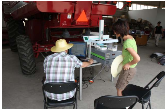
Figure 3. After the water vapor isotope measurements had concluded, the analyser was set up in a building adjacent to the cornfield studied in the Beijing field campaign and was used to quantify the isotopes in liquid water samples provided by the participants from their home countries.
