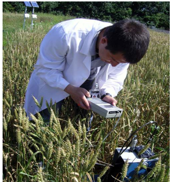
Photo 1. Estimating the soil water in the wheat field using the neutron moisture sensor.
