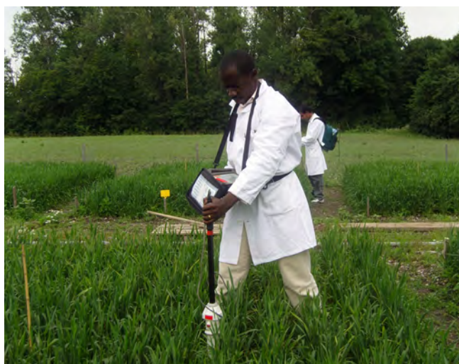
Fellows monitoring soil water in the field using a time domain reflectometer.
