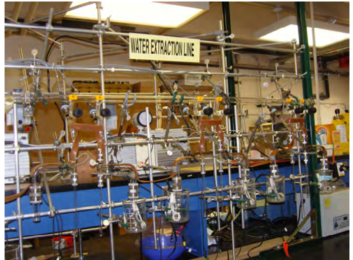
A cryodistillation water extraction line at the Stable Isotope Facility Laboratory, University of Wyoming, WY, USA.
