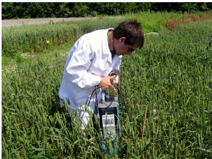
Monitoring soil water in the field using a soil moisture neutron probe
