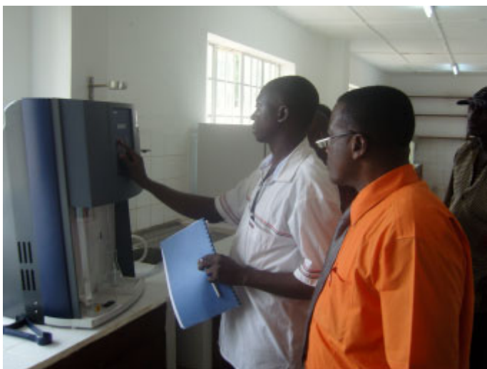
Photo 3. A former fellow demonstrating the use of Kjeldhal distillation equipment for nitrogen analysis at the Soils Analytical Laboratory at the Agricultural Research Station, Rokupr, Sierra Leone.
