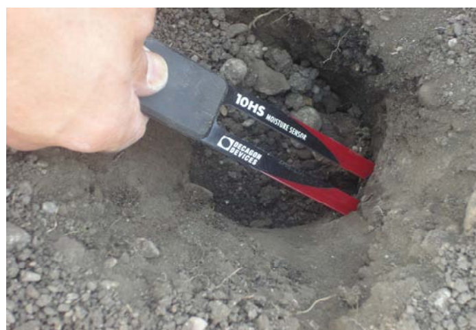
Photo 2. The new soil moisture device 10HS being installed on the field.
