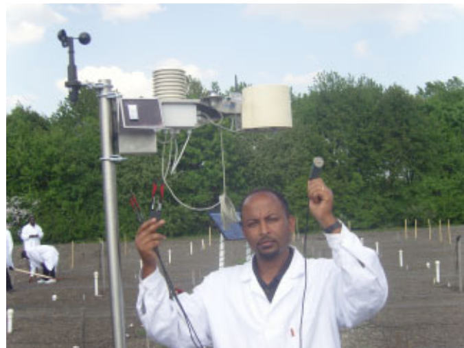
Photo 1. The imetos weather station and Decagon soil moisture sensors to be installed in the field at the Agency's Laboratory Seibersdorf.
