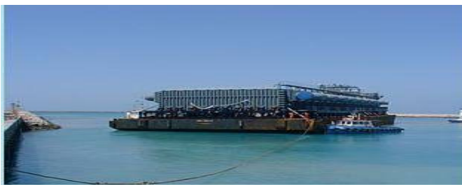
MSF-Desalination unit on barge, Al-Taweelah, UAE
