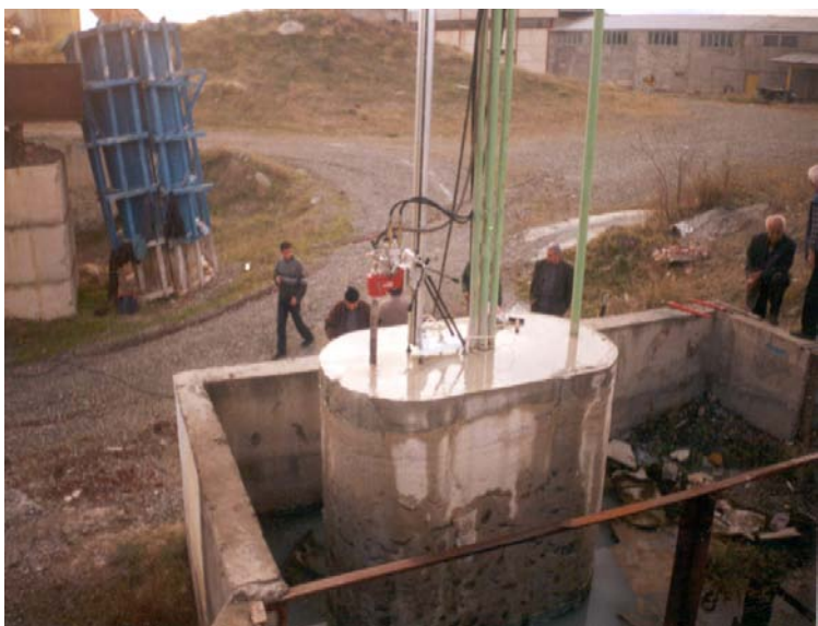
Mock-up testing of entombment concept for reactors, conducted in Georgia
