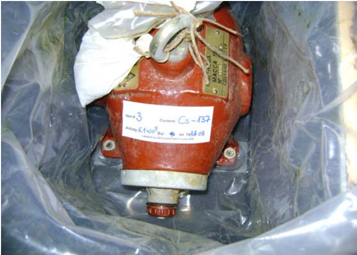
Identified and labelled gauge housing a CS-137 source
