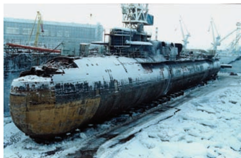
Dismantling a Delta-class submarine at the Zvezdochka shipyard in Severodvinsk, RF
