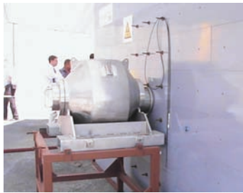
View of the Long-Term Storage Shield mated to the Hot Cell pass-through port
