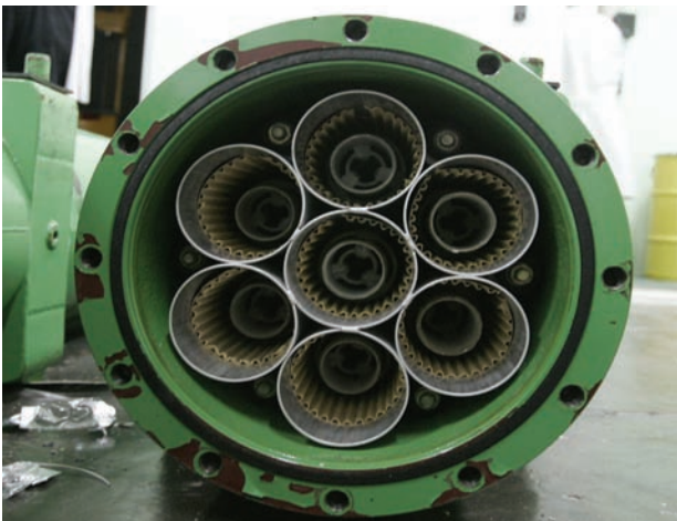
Shipping container filled with fresh HEU Fuel
