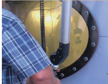
Manipulating the 2000 Ci source during testing.
