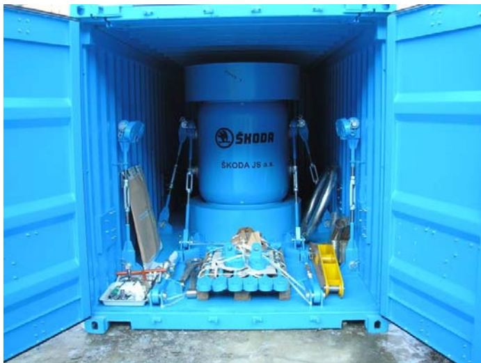
A Spent Nuclear Fuel Transport and Storage System including cask, ISO container and all related tooling; purchased through RER/4/028.
