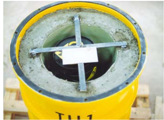
A waste-container with shielded waste ready for sealing
