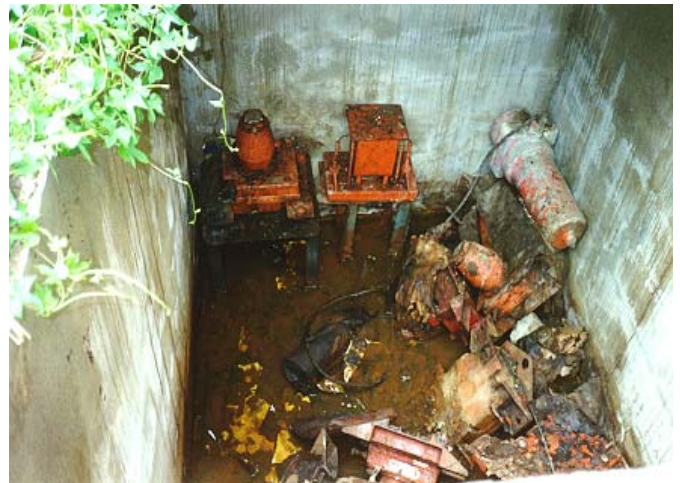
Inappropriate storage of disused sealed radioactive sources
