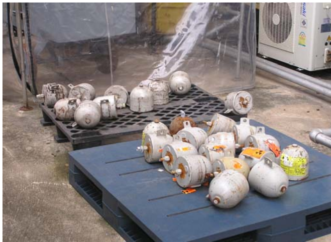
Sealed sources being prepared for conditioning
