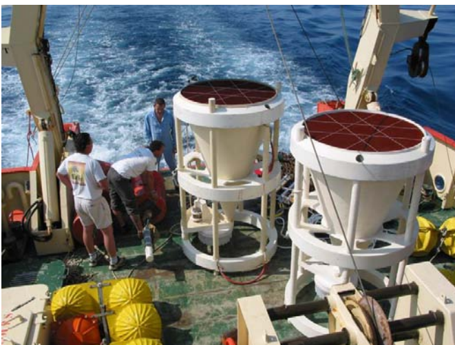
Figure 4: Sediment traps (1 m 2 collection surface) Technicap PPS5 used to collect carbon containing sinking particles in the NW Mediterranean.
