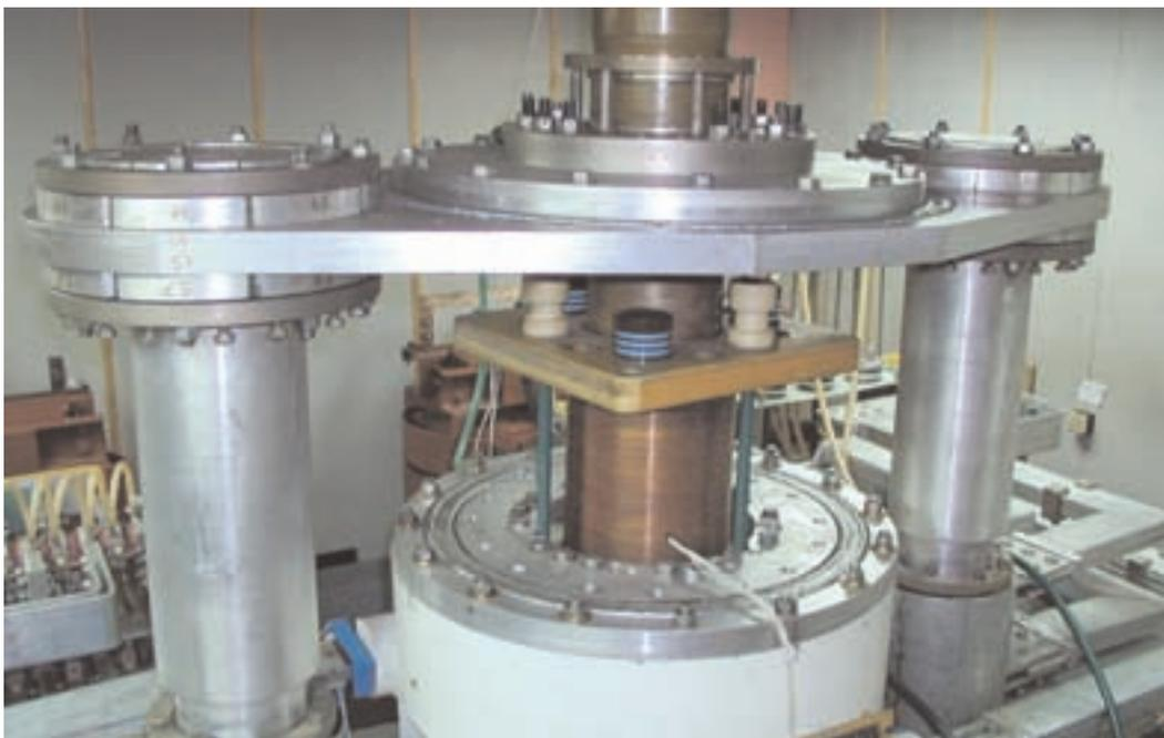
*Figure 5. Thermal test of the protective breaker with water-cooling under steady-state current 70 kA.*
