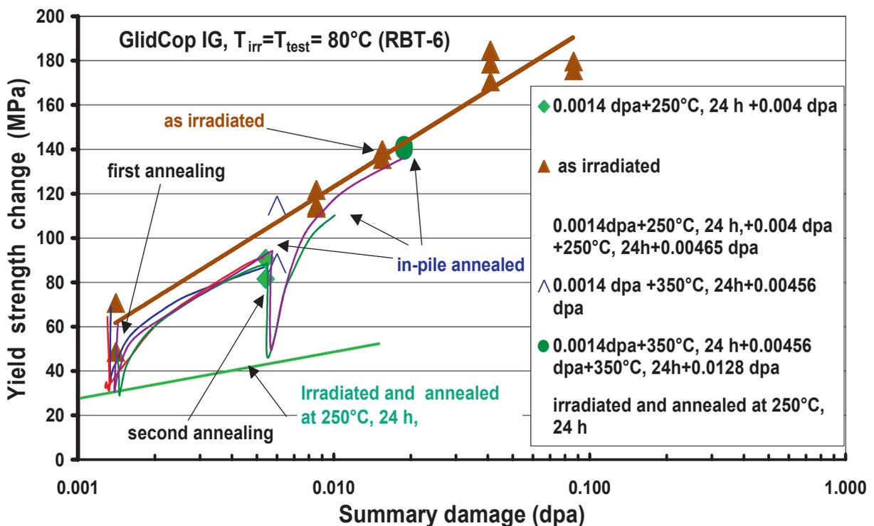
Figure 4. Change in the yield strength plotted versus neutron damage for GlidCopAl25IG alloy: as irradiated; annealed after irradiation at  $250^{\circ}\text{C}$ , 24 h; after IAI cycles.
