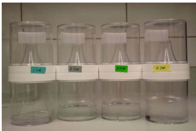
Experimental set-up to study the effect of water depth on Aedes albopictus larvae.
