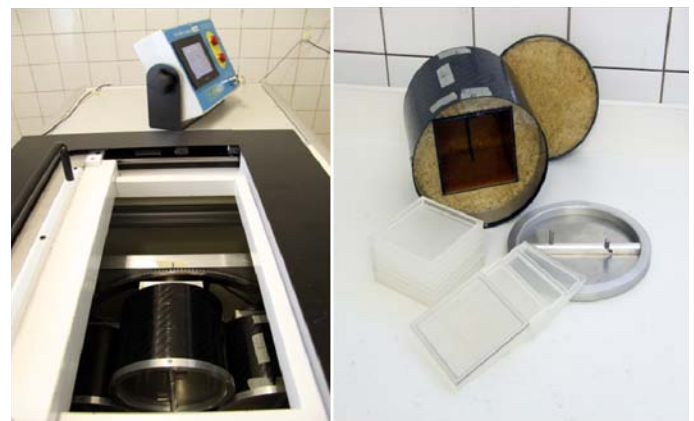
The opened chamber of the RS 2400 X ray irradiator holds 5 rotating cylinders (left side), which have been modified for the irradiation of mosquito pupae.
