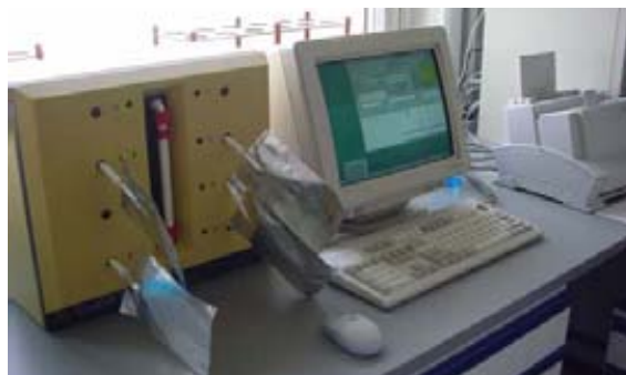
Figure 3. Laser based system for breath test analysis.
