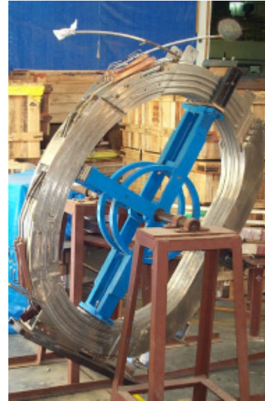
FIG. 2. A picture of SST-1 TF coil
