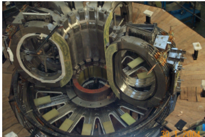
FIG. 5. TF modules on the support beams
