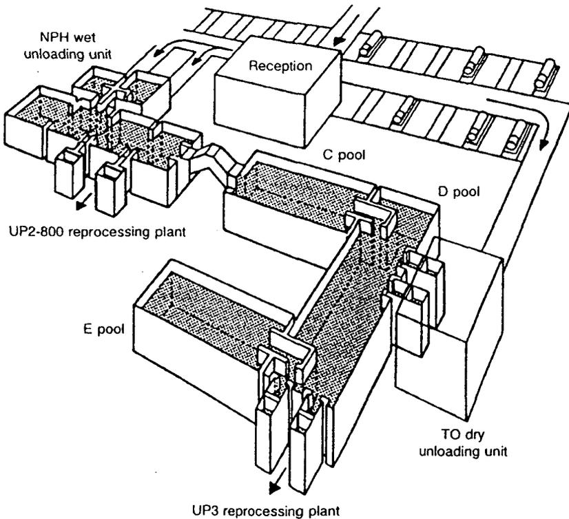
FIG. 15. Spent fuel reception, unloading and storage complex at La Hague, France.
