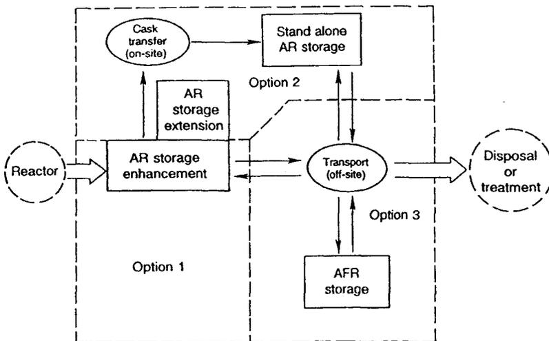
FIG. 3. Three options for the storage of spent fuel (arrowed lines are possible transport operations).
