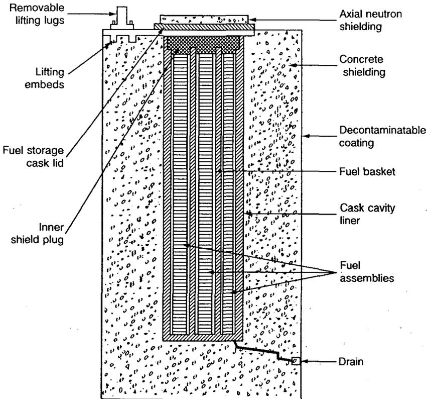
FIG. 7. Conceptual design for an unventilated concrete storage cask.
