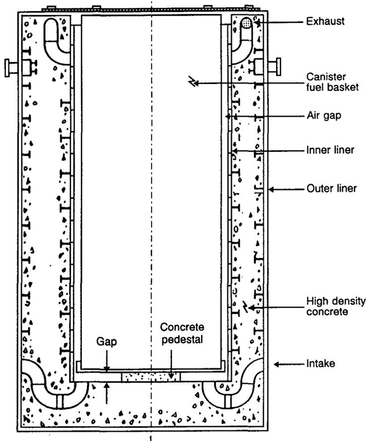
FIG. 8. Conceptual design for a ventilated concrete storage cask.
