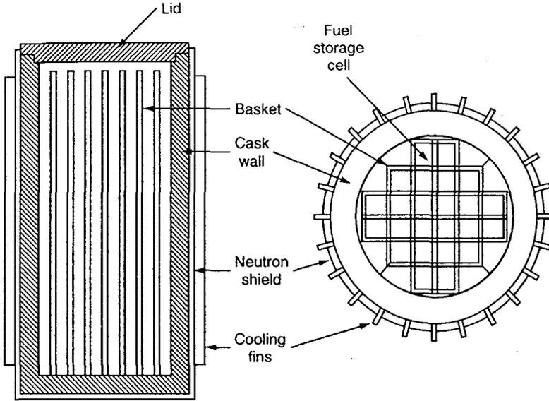
FIG. 6. Conceptual design for a typical metal storage cask.
