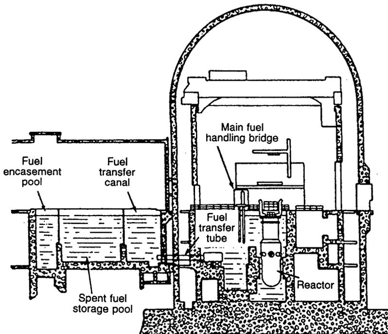
FIG. 5. Cross-section showing the relationship of the PWR core and the spent fuel pool.
