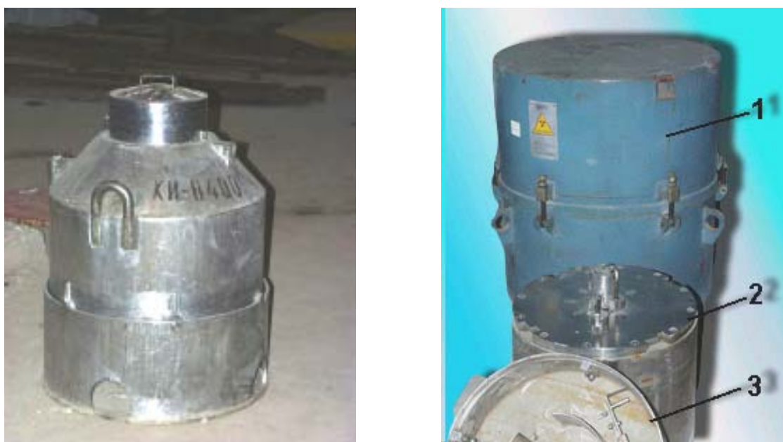
FIG. C-2. Standard containers for transportation and storage of sealed radioactive sources. Left – Container KI-8400. Right – transport complex UKT1B:1 – casing, 2 – container KROT-100, 3 – transport casing lid.
