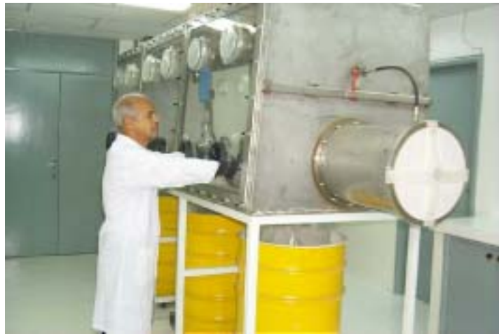
FIG. C-7. Glove box for ^{241}\text{Am} lightning rod dismantling.
