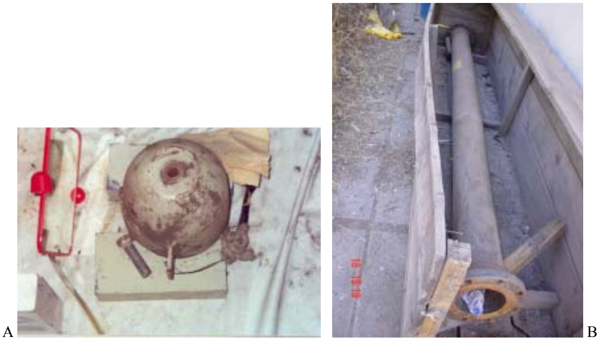
FIG. 8. A photograph of two large size disused long lived sources. A) Source in form of a large shielded process control source in a coal fired power plant. B) Source with a long active tube (within the large tube with flanges at both ends).
