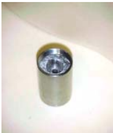
FIG. C-3. Prefabricated stainless steel capsule for immobilisation of Ra-226 sources. A: The capsule is opened for location of source into the conical socket. B: The capsule is sealed for emplacement into transportation and storage container.
