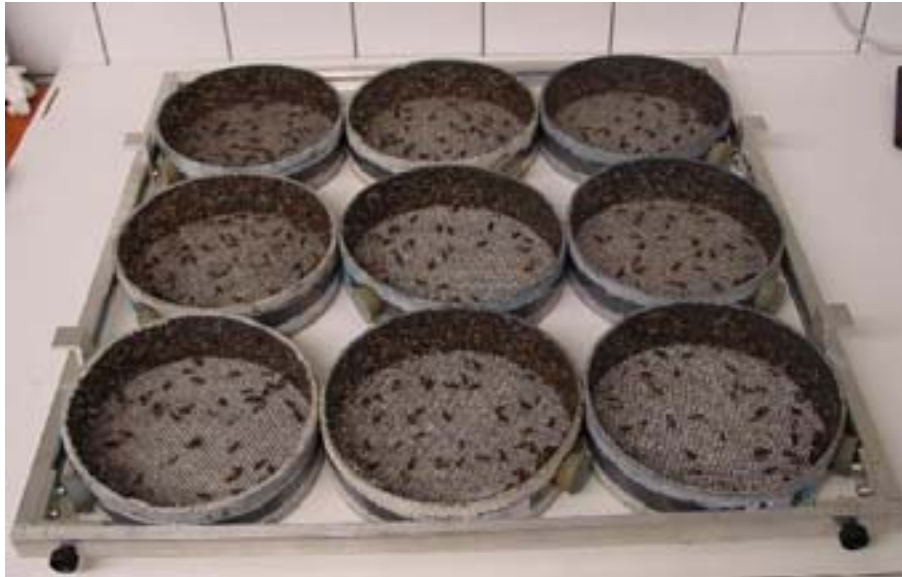
Figure 10. Standard 200 mm diameter cages in a holding frame for the TPU 3 system.
