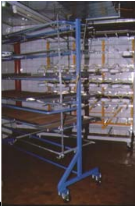
Figure 5. Tsetse Production Unit 2. (a) Cage holding frame, with 7 levels of 9 cages each. (b) Pupal collection unit. (c) Rear of cage holding frame to show the lever system to lower the cages onto the feeding membranes.
