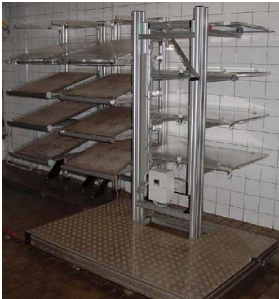
Figure 9. Prototype tsetse production unit 3 (TPU 3). Two holding units are shown on the left and a feeding unit on the right.
