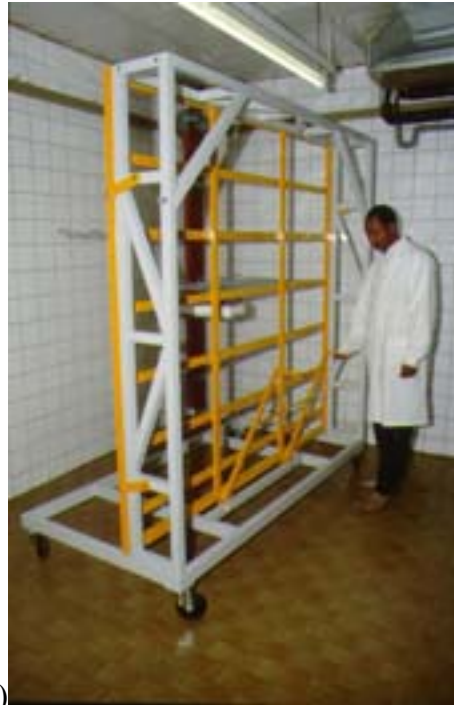
Figure 5. Tsetse Production Unit 2. (a) Cage holding frame, with 7 levels of 9 cages each. (b) Pupal collection unit. (c) Rear of cage holding frame to show the lever system to lower the cages onto the feeding membranes.
