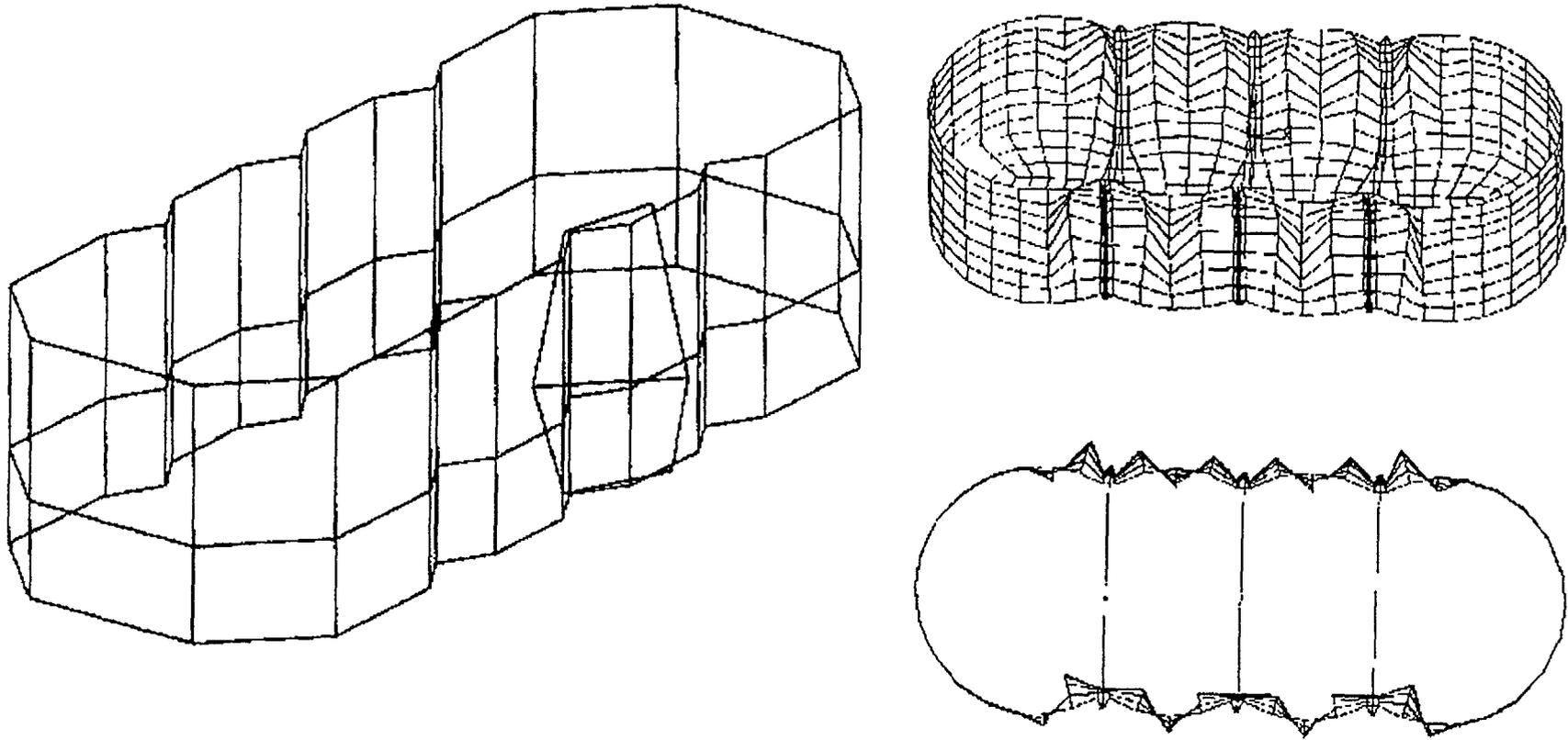
Figure 7 Comparison of the calculated and defined by the full scale tets mode shapes (calculated natural frequency for 1.3 scale model 20 752 Hz, for 1 1 scale 7 437 Hz, experimental value 7 52 Hz)
