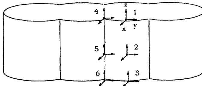
Figure 1 Location of the acceleration sensors on the worm-tank
