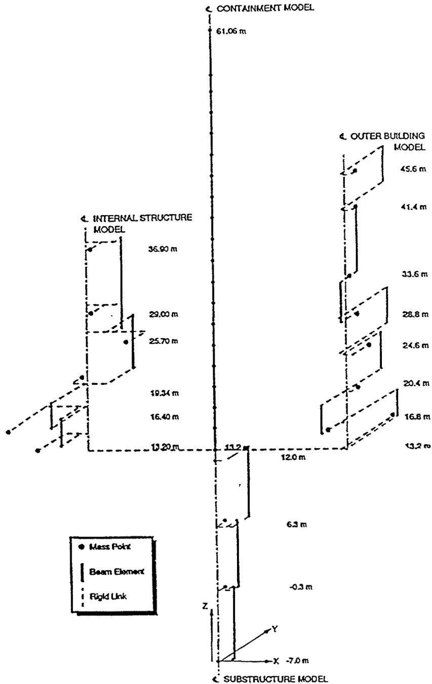
Fig. 3.1 Kozloduy 1000 MW Unit Beam Element Model
