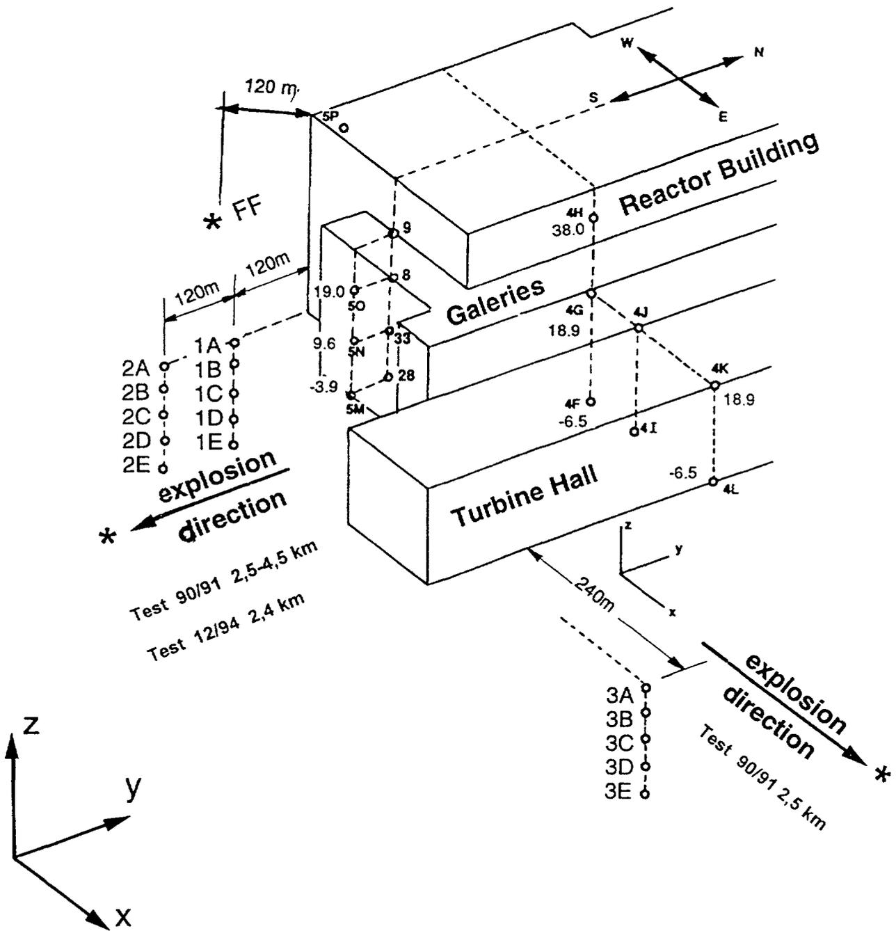
Fig. 4 PAKS Nuclear Power Station Site Arrangement of Measuring Points (2<sup>nd</sup> Series of Experiments)
