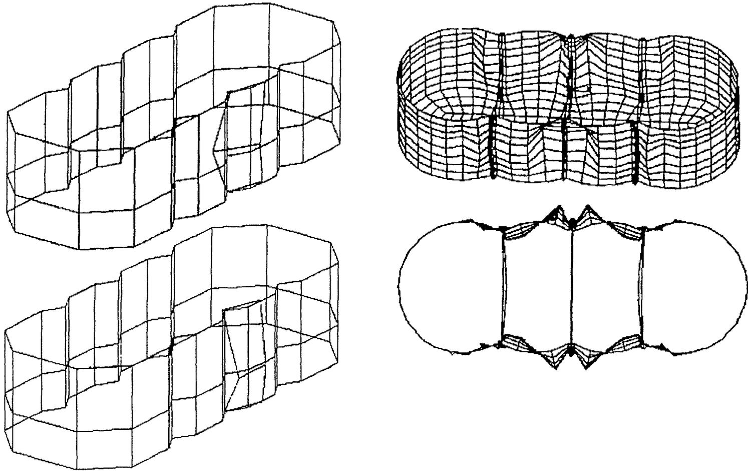
Figure 8 Comparison of the calculated and defined by the full scale tests mode shapes (calculated natural frequency for the 1/3 scale model 26.6 Hz, for 1/1 scale 9.37 Hz, experimental value 9.37 Hz)
