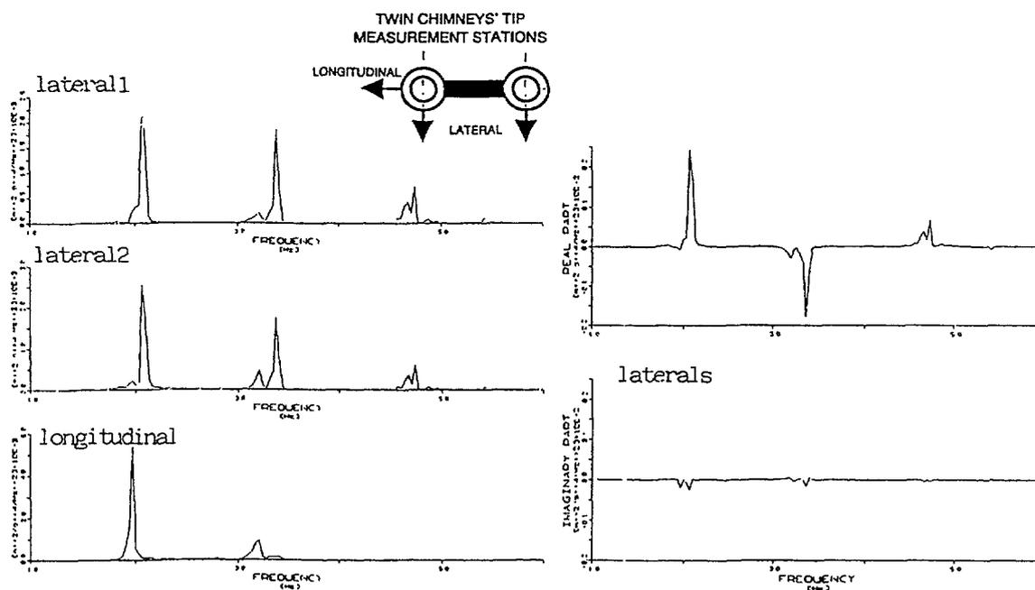
Figure 7. Energy auto-spectral densities of the twin chimneys' tip transverse and longitudinal responses
