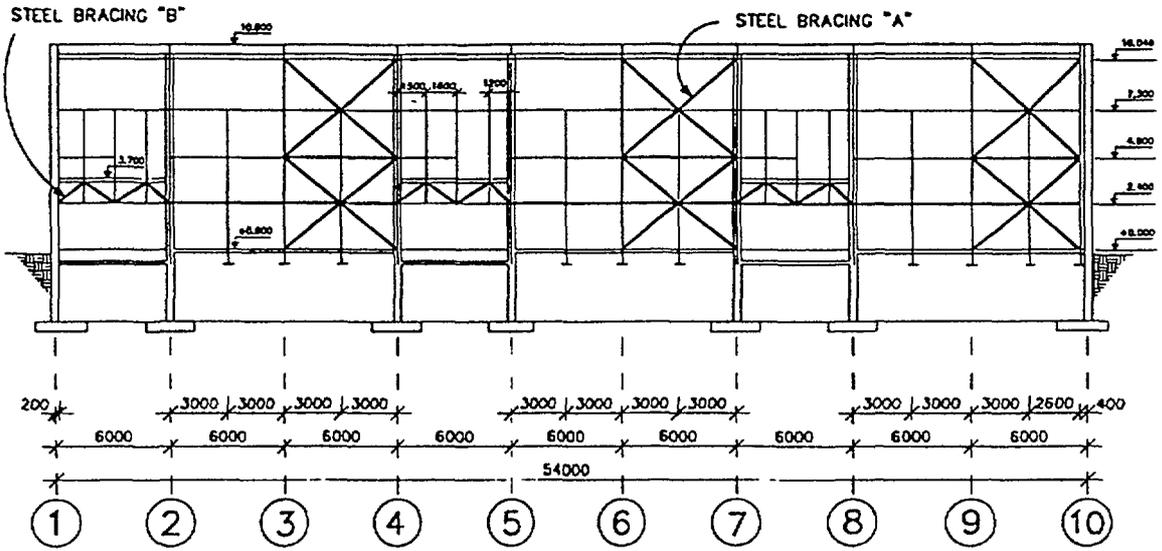
Figure 11: Exterior Wall Elevation At Line "A", Looking South
