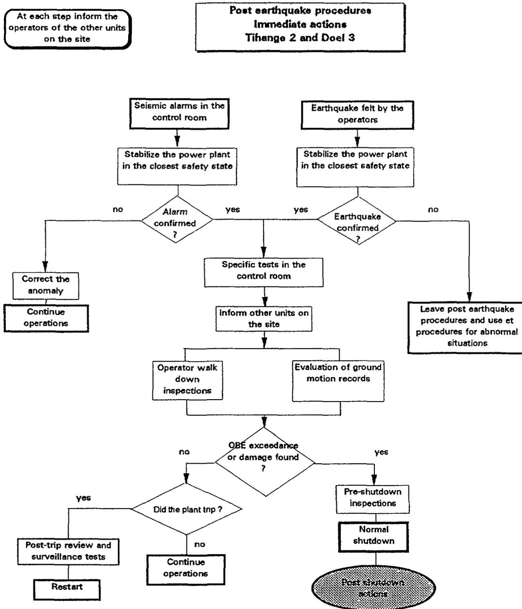
**Figure 4 - Post earthquake immediate Actions**
