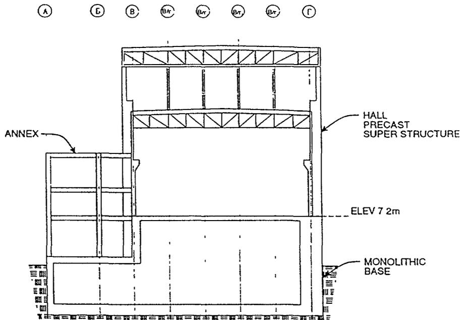
Figure 2 Vertical Cross Section at Axis 7
