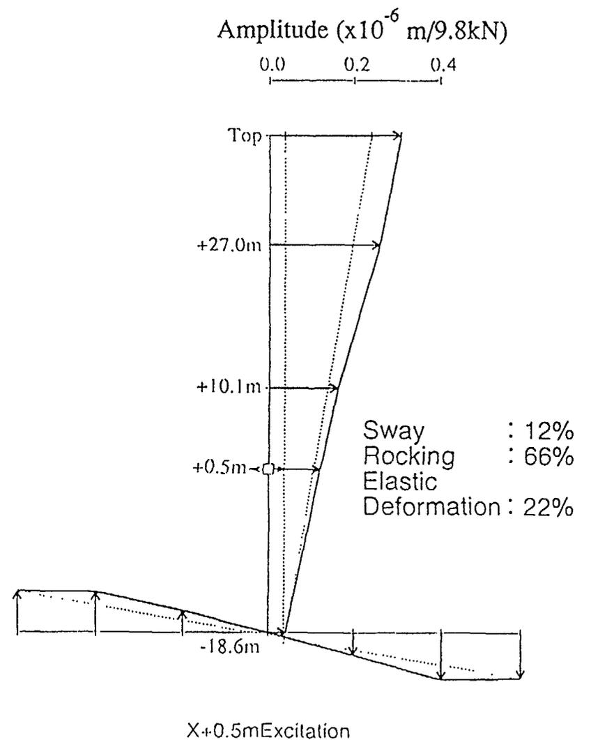
Fig.5 Vibration mode shapes of Atucha II reactor building ( $f=3.5\text{Hz}$ )
