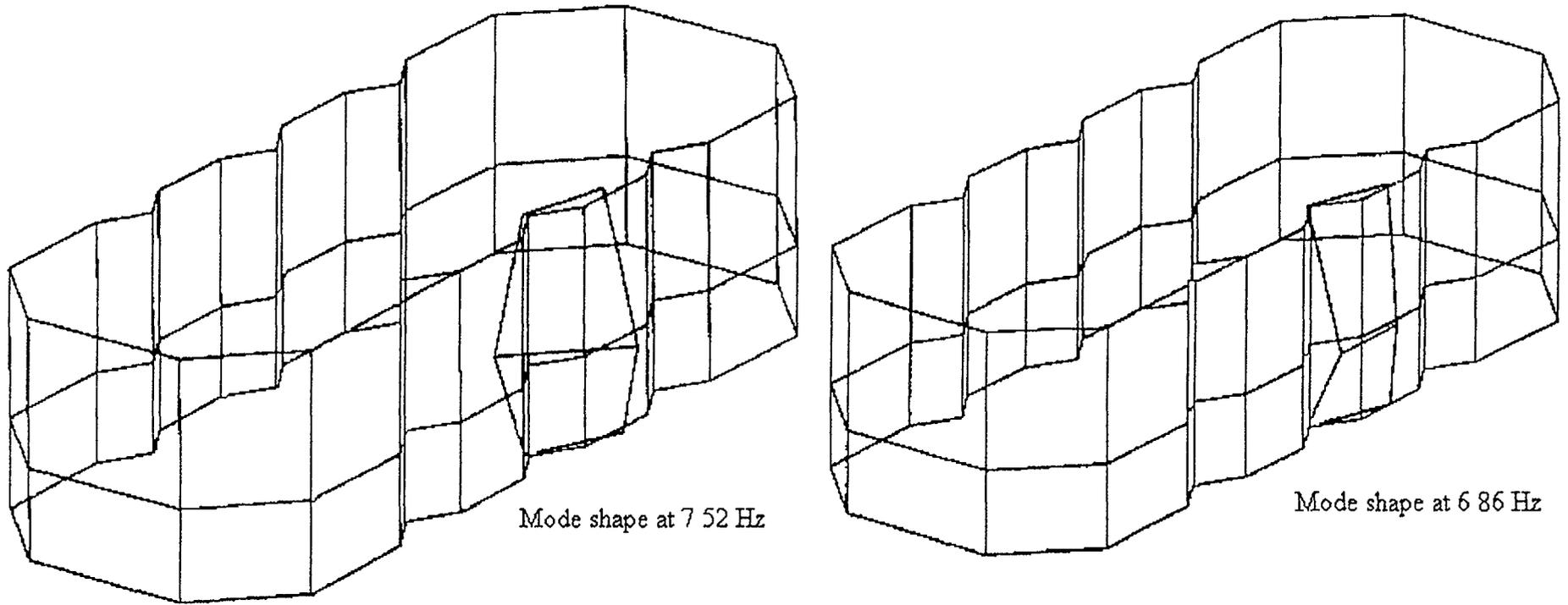
Figure 4 Mode shapes defined from the full scale tests
