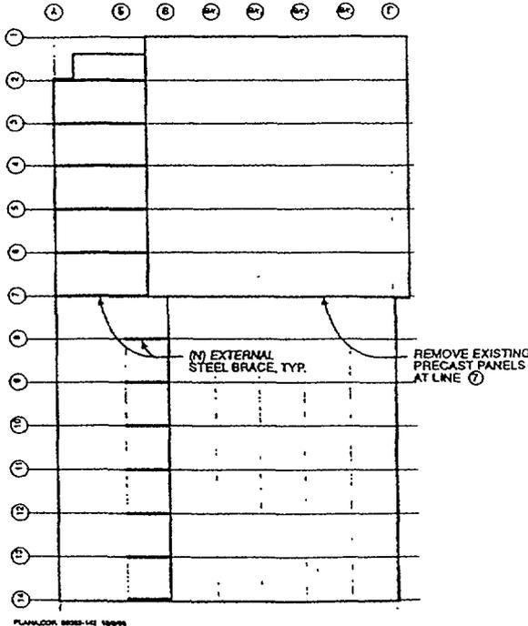
Figure 7 Plan of Structural Upgrades at Roof Level
