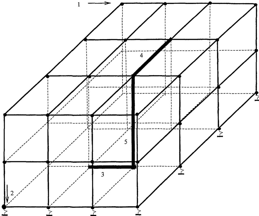
Figure 10. Beam model of auxiliary building concrete block
