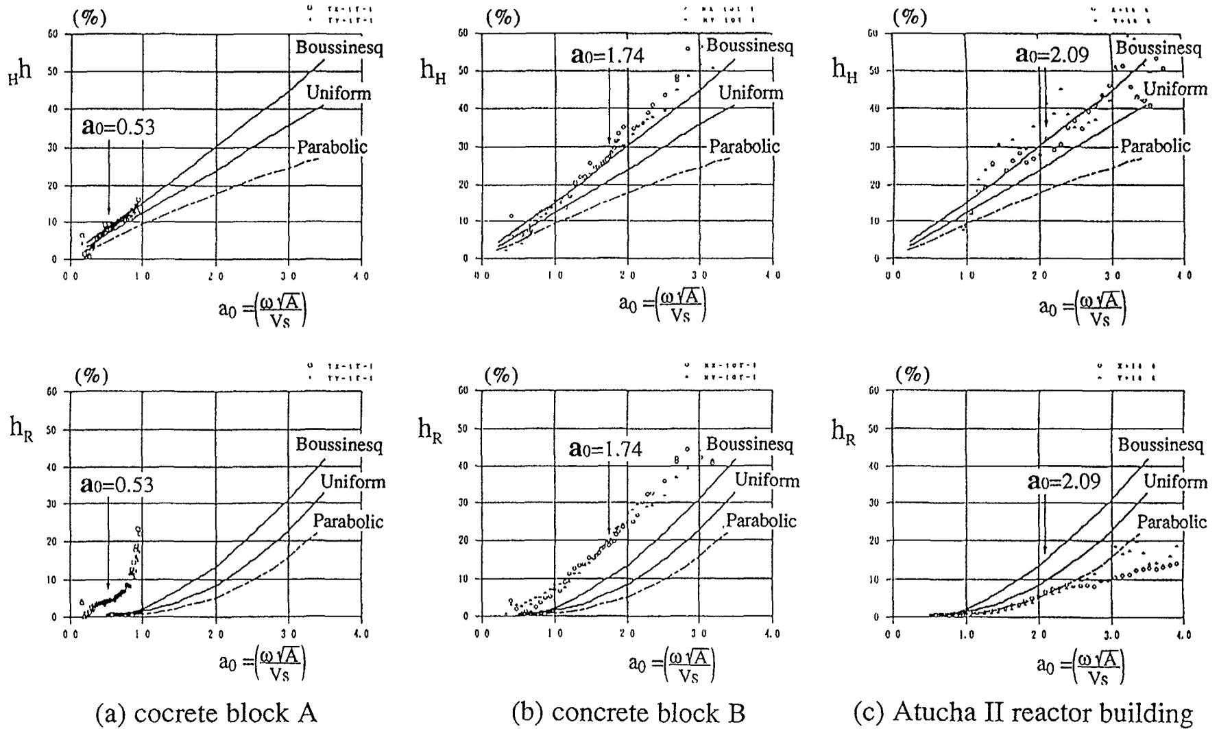
Fig.18 Damping constants of concrete block A, block B and Atucha II reactor building comparing with the test results and the theoretical value by vibration admittance
