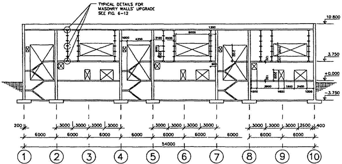
Figure 12: Exterior Wall Elevation At Line "B", Looking South
