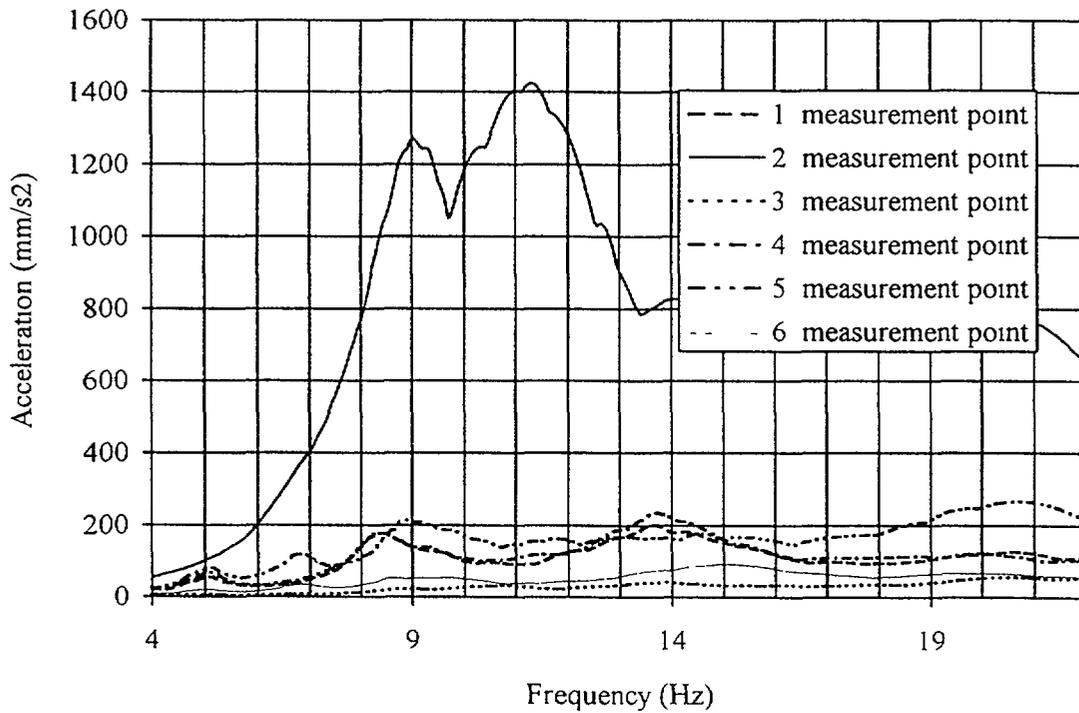
Figure 2 Examples of the test evaluation results plots of the response spectra for the different points on the worm-tank
