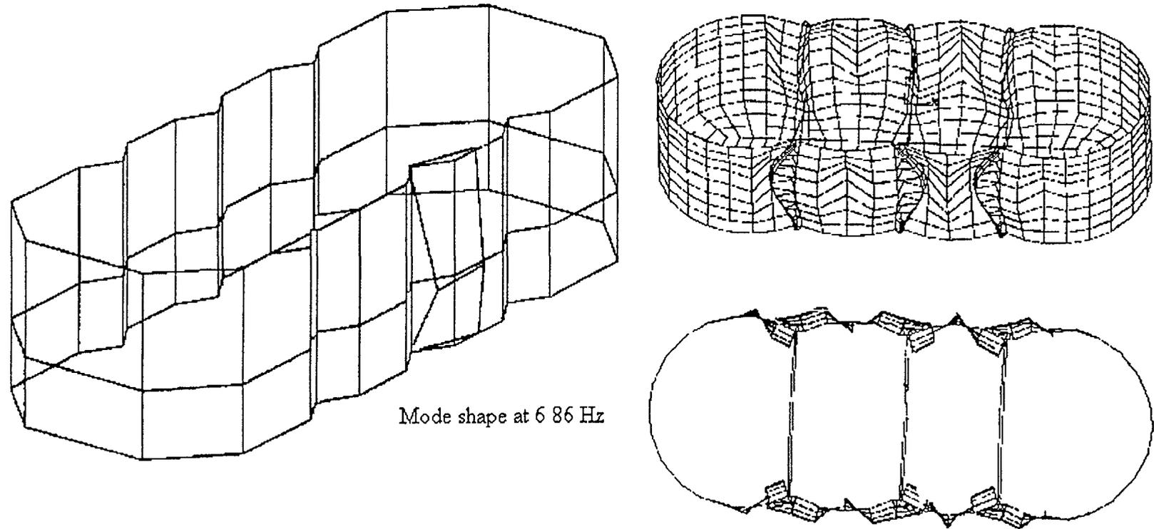
Figure 6 Comparison of the calculated and defined by the full scale tests mode shapes (calculated natural frequency for 1/3 scale model 21 656 Hz, for 1/1 scale 6 981, experimental value 6 86 Hz)
