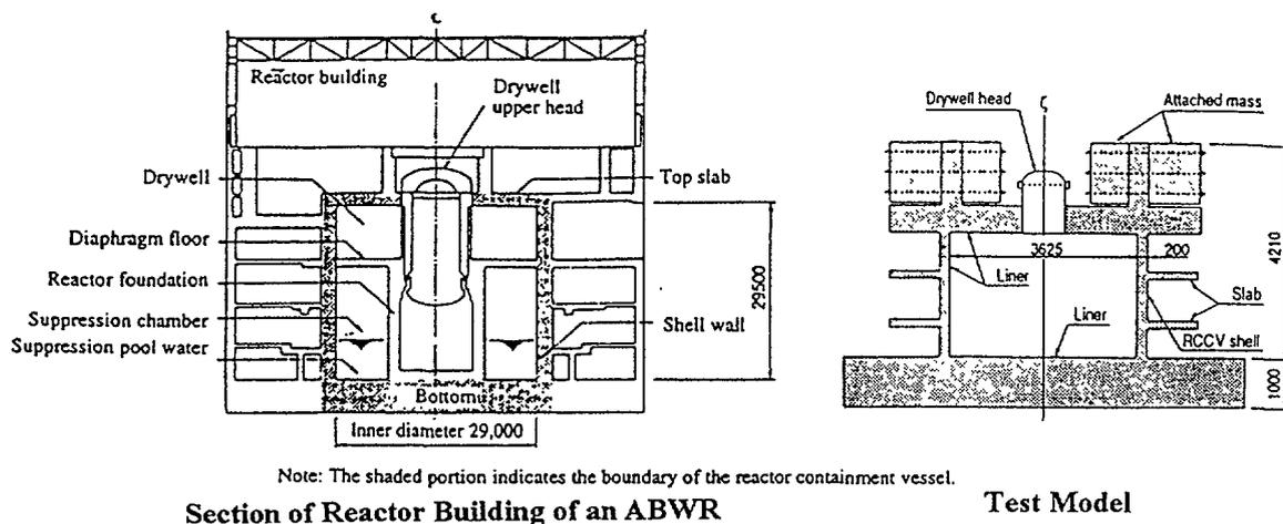
Fig.7 An Outline of Actual RCCV and a Scaled Test Model in Planning.
