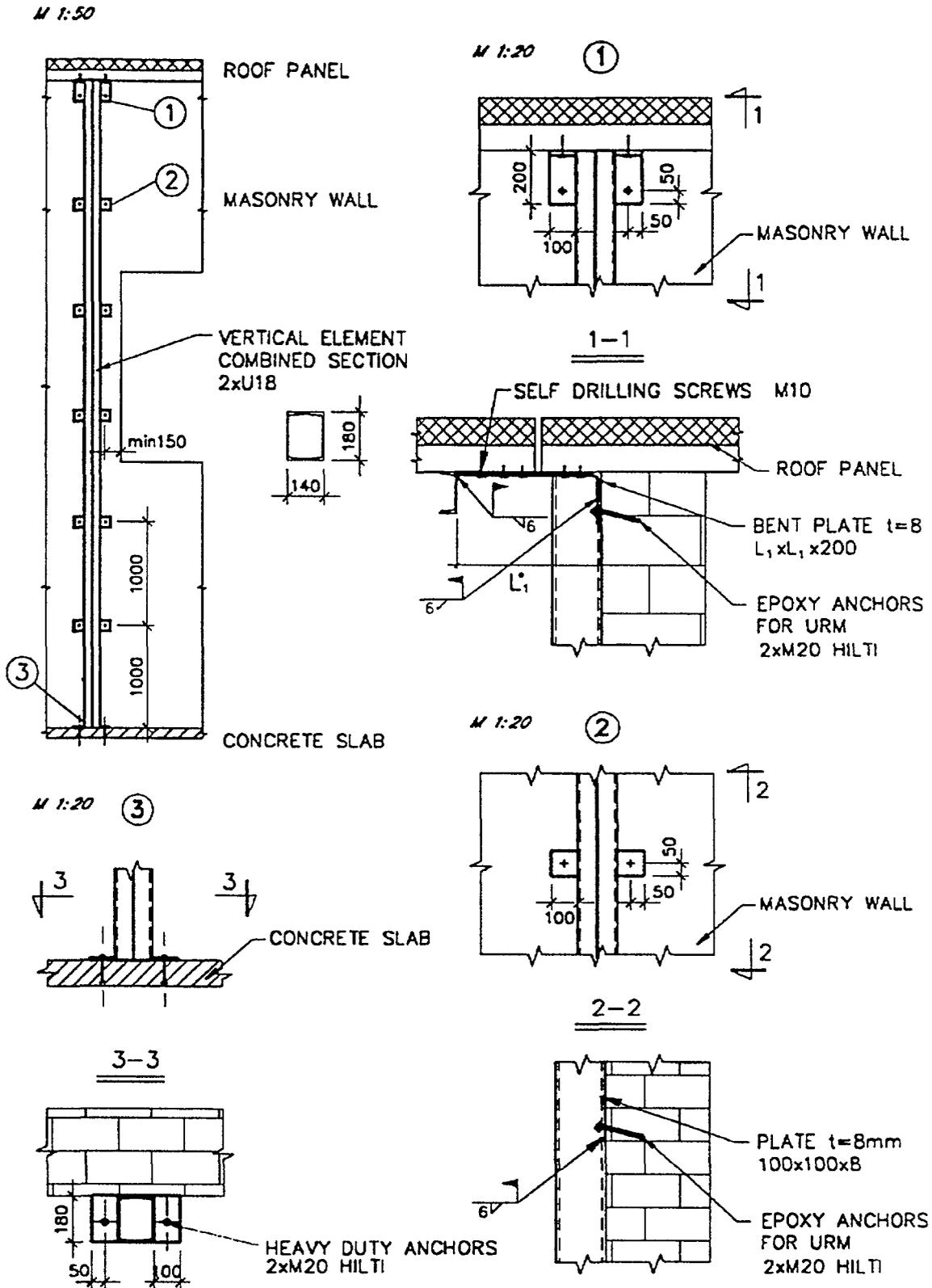
Figure 13: Typical Details for Masonry Walls' Upgrade
