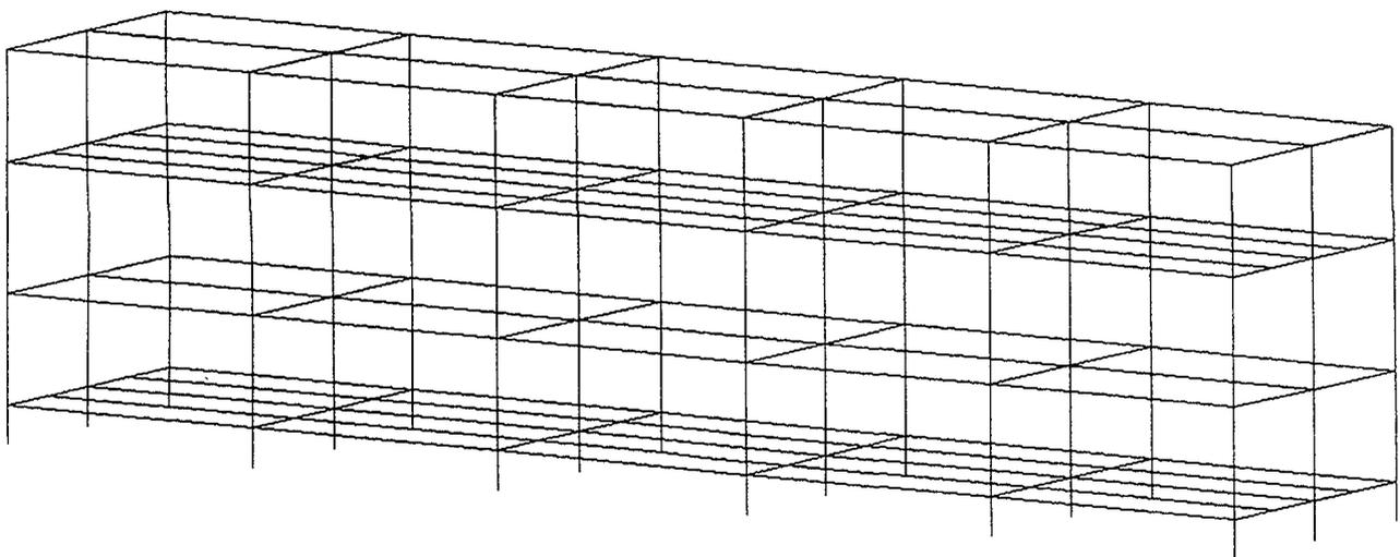
Fig. 6 3D FINITE ELEMENT MODEL OF BATTERY RACKS FOR KANUPP
