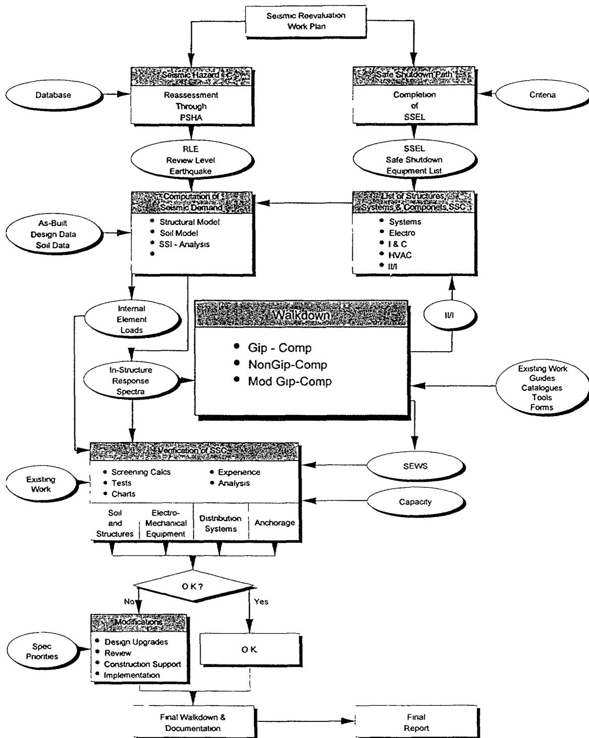
Figure 1: Flowchart for Seismic Verification of SSCs
