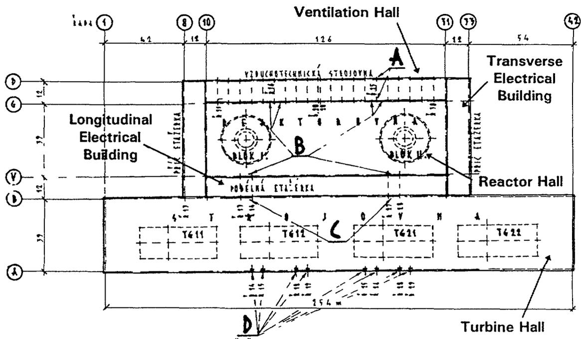
Figure 2: Reactor Building Complex Plan View
