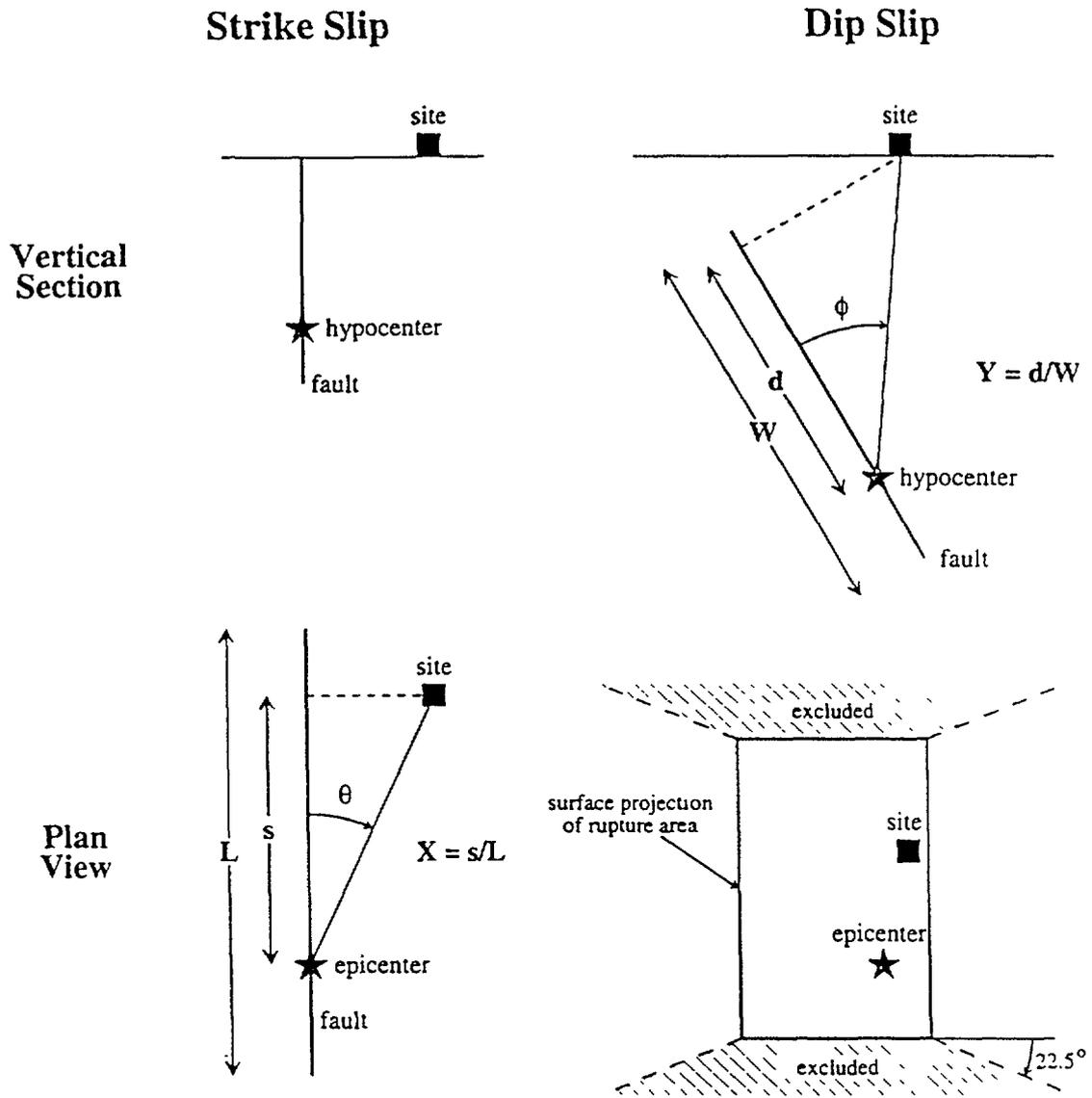
Fig 9 Definitions of rupture directivity parameters (Somerville 'et al', 1997)
