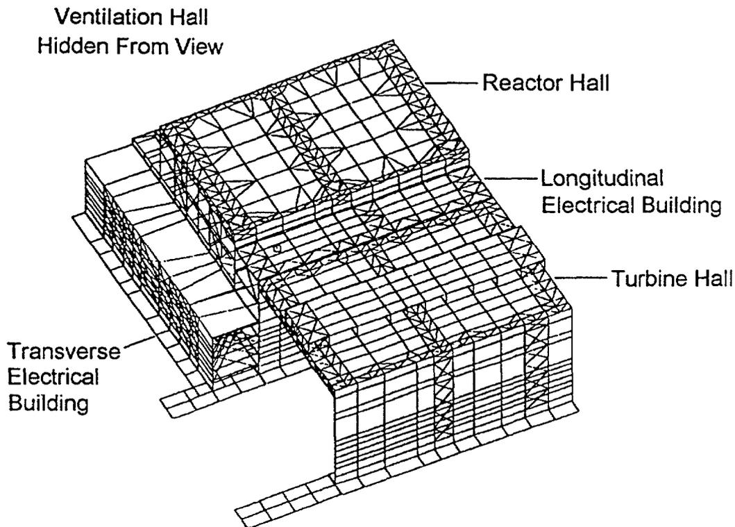
Figure 3: SASSI Structural Model of Reactor Building Complex
