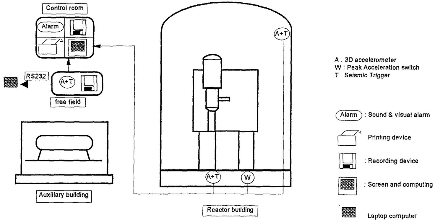
Figure 7 - TIHANGE and DOEL New Seismic Instrumentation
