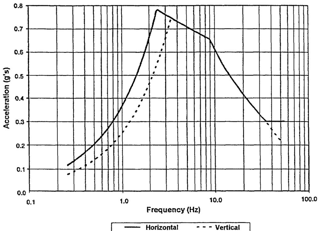
Figure 1: iRLE Ground Response Spectrum
