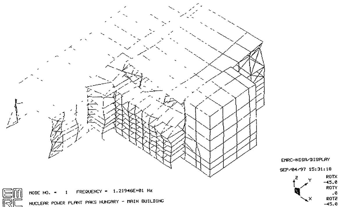
Figure 2. Deformed shape - example of mode n1.
