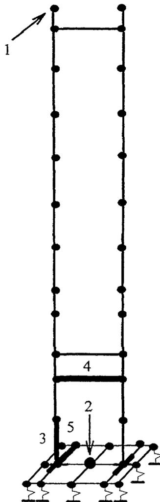
Figure 4. Beam model of ventilation chimney
