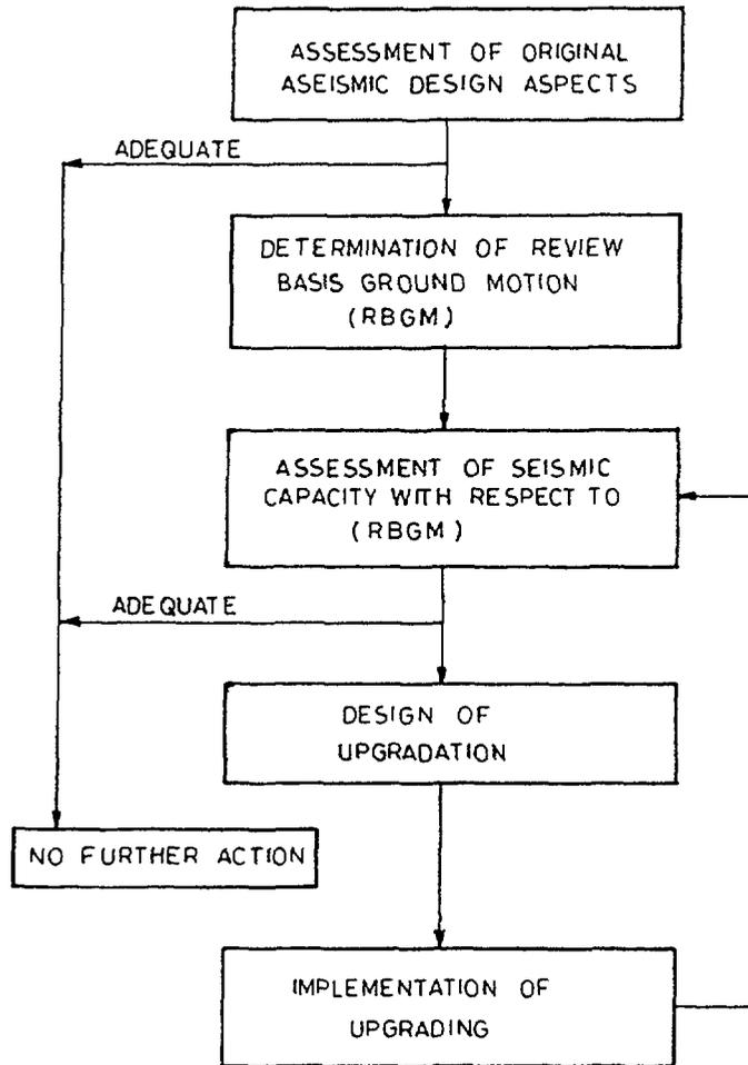
*FIG. 2. Flow diagram for seismic qualification of existing nuclear installations (following proposed method).*
