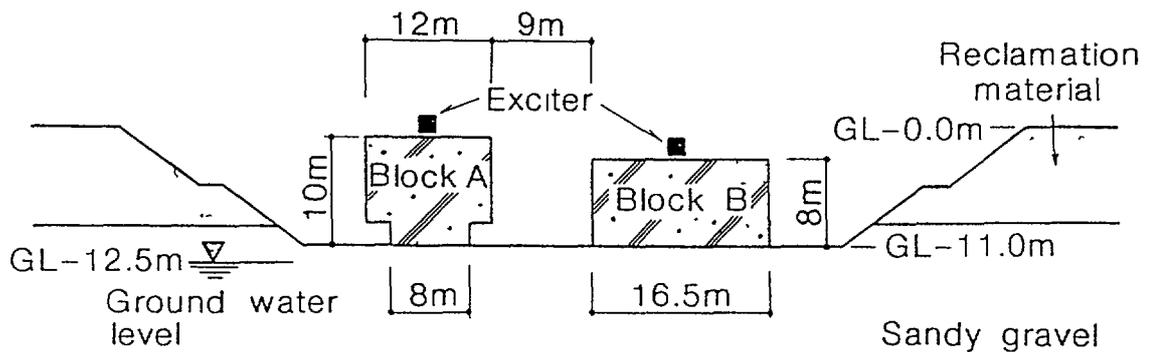
Fig.7 Concrete blocks A and B constructed on the test ground
