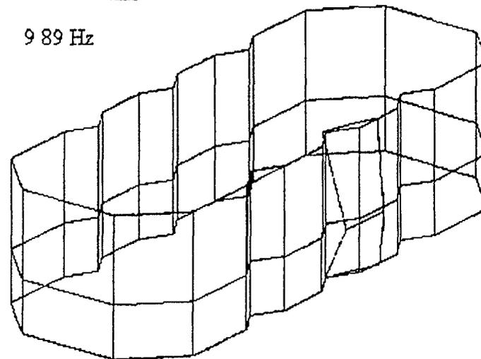
Figure 5 Mode shapes at 8 63 and 9 89 Hz defined from the full scale tests
