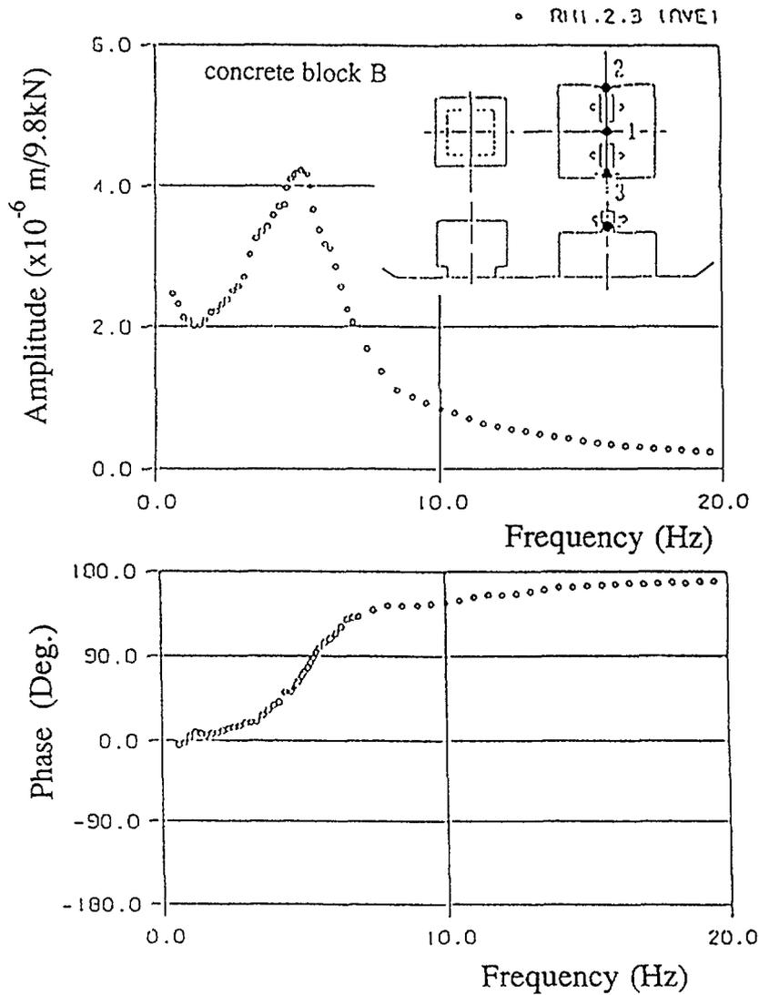
Fig.9 Resonance and phase lag curves of concrete block B
