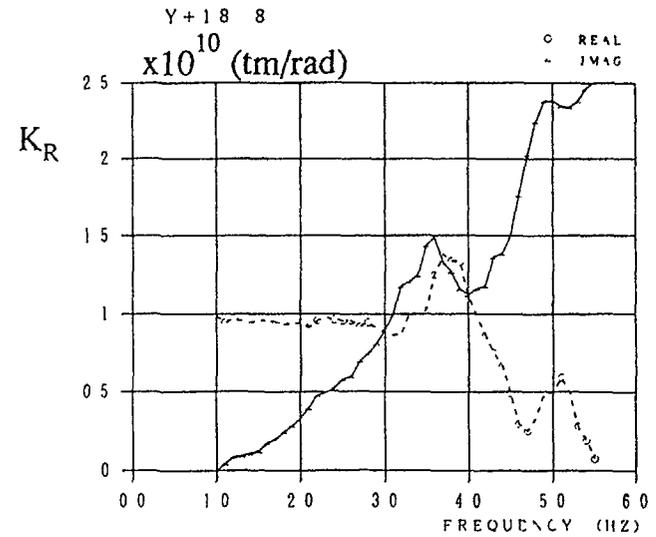
Fig 10 Soil springs concentrated at the basemat bottom of Atucha II reactor building derived by back fit analysis (X direction excitation)
