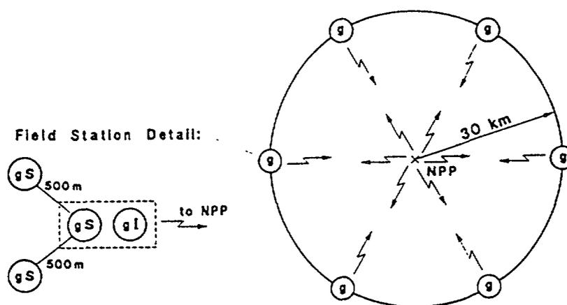
Fig. 1 Layout of seismic monitoring system of Ignalina nuclear power plant (NPP)
