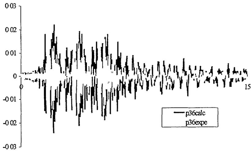
Figure 13 Calculated and measured responses for point P36
