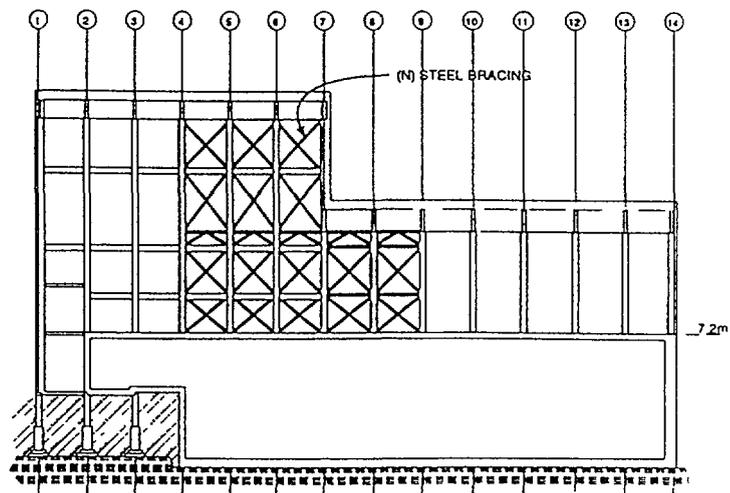
Figure 5 Longitudinal Vertical Steel Braces
