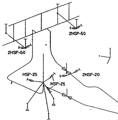
Figure 4 Snubber Location for Loop No 1 of PCLS
