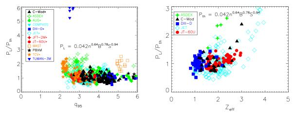
Fig. 5. Measured H-mode threshold power normalized to that of Eq. 3 vs.  $q_{95}$  showing a trend to increase the relative threshold power for  $q_{95} < 3$ .
