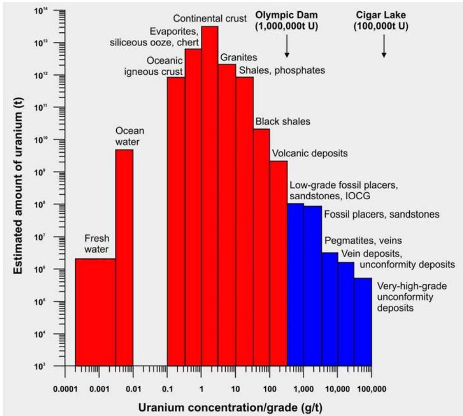
FIG. 25. Uranium distribution in the earth's crust. Data source: Ref. [93]. Note: IOCG: iron oxide copper gold (deposits).
