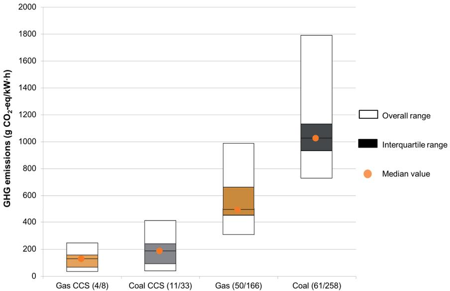
FIG. 3. Life cycle GHG emissions from electricity generation: fossil fuels and carbon capture and storage. Data source: IAEA [17]. Note: The numbers in parenthesis indicate the number of sources/estimates. The interquartile range includes half of the calculations around the median of the overall range. CCS – carbon capture and storage.
