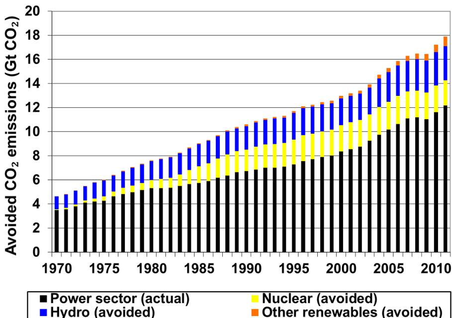
FIG. 5. Global CO<sub>2</sub> emissions from the electricity sector and emissions avoided by using three low carbon generation technologies. Data source: Ref. [19].
