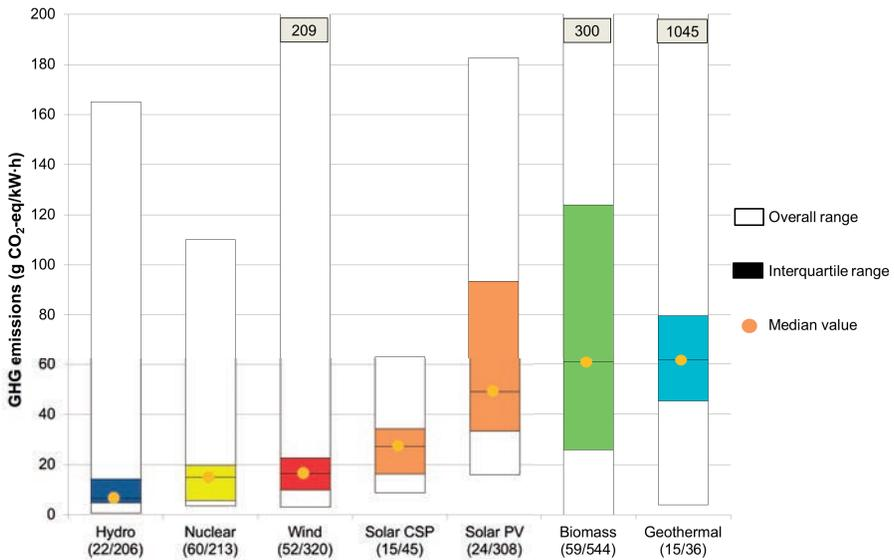
FIG. 4. Life cycle GHG emissions from electricity generation: renewable technologies and nuclear power. Data source: IAEA [17]. Note: The numbers in parenthesis indicate the number of sources/estimates. The interquartile range includes half of the calculations around the median of the overall range. CSP — concentrated solar power; PV — photovoltaic.
