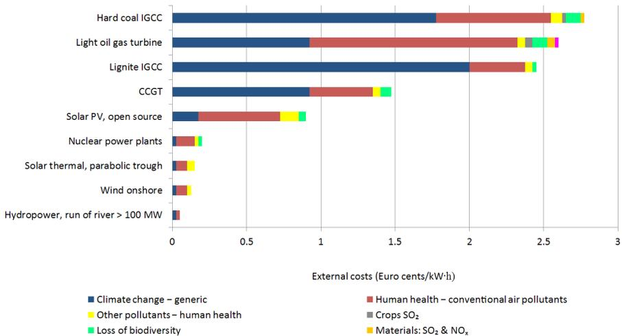
FIG. 18. Estimated average external costs in the EU for selected electricity generation technologies between 2005 and 2010. Data source: Ref. [45]. Note: IGCC — Integrated Gasification Combined Cycle, CCGT — Combined Cycle Gas Turbine.
