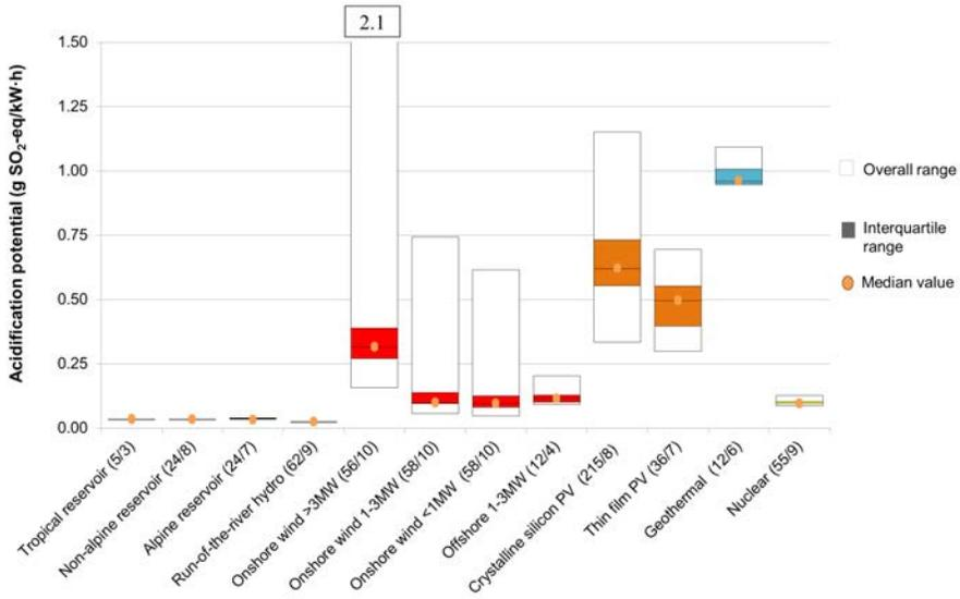
FIG. 17. Acidification potentials of emissions from renewable and nuclear technologies in g SO<sub>2</sub>-eq per kWh by type of technology. Data source: Ref. [15]. Note: The interquartile range includes half of the calculations around the median of the overall range.
