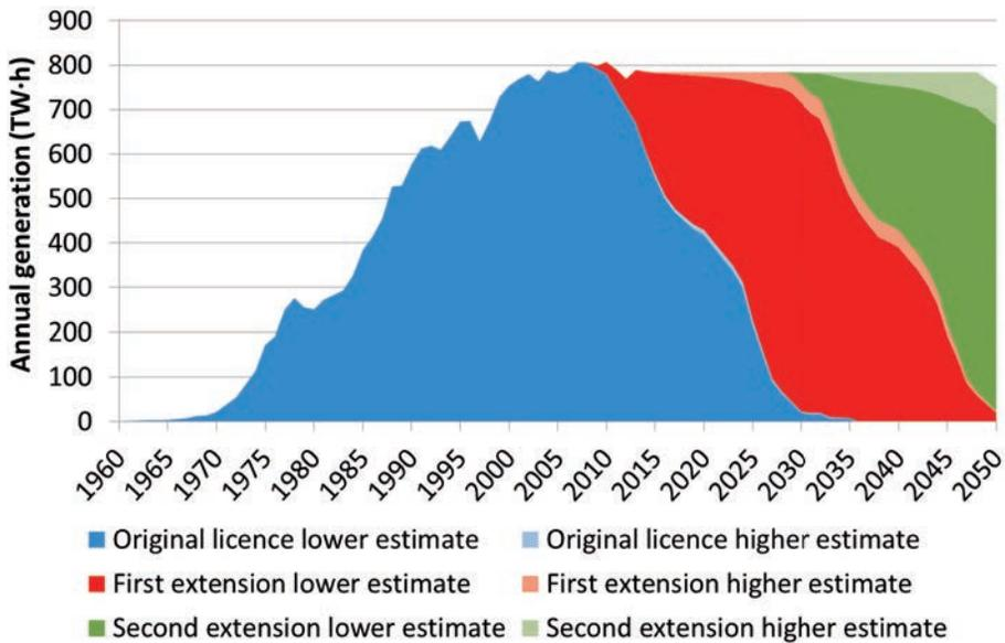
FIG. 34. Historical and projected nuclear electricity generation from the USA's current nuclear fleet under different assumptions for lifetime extensions.
