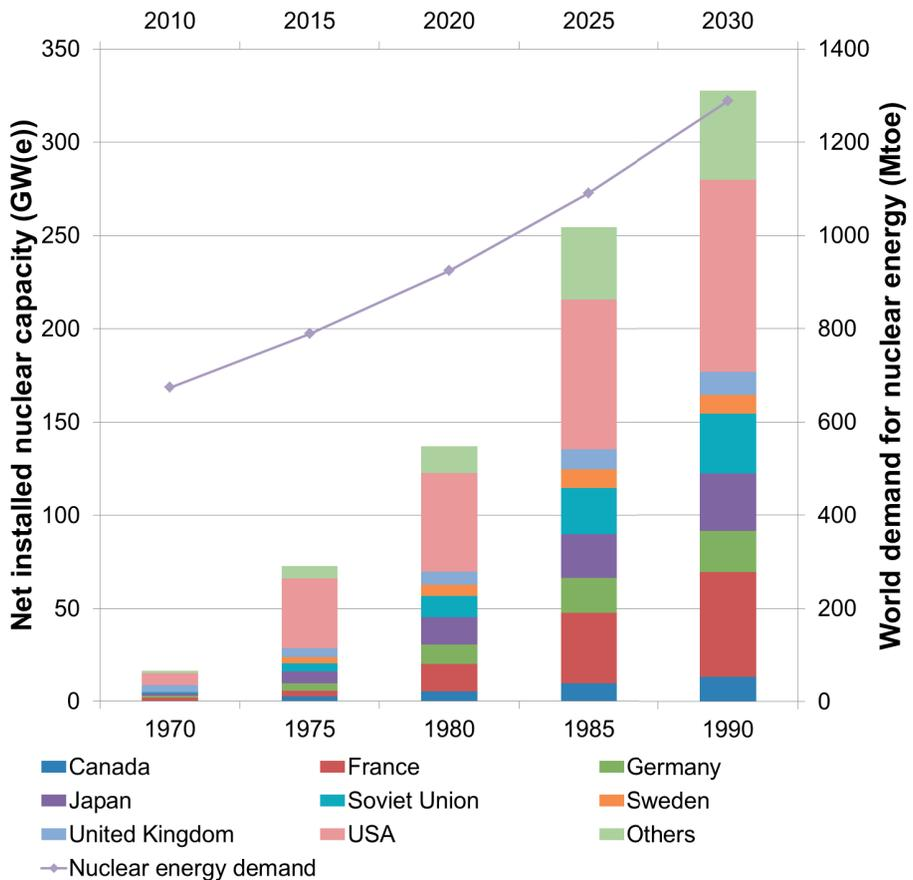
FIG. 24. Net installed capacity of the nuclear industry (GW(e)) in 1970–1990 (left vertical and lower horizontal axis) and projected expansion of world primary energy demand for nuclear energy, according to the IEA 450 Scenario in 2010–2030 (right vertical and upper horizontal axis). Data sources: Refs [8, 13, 81, 82].
