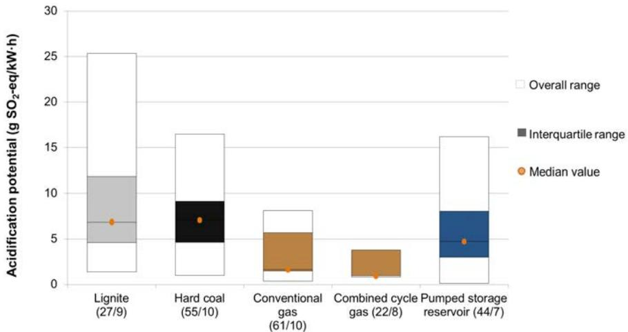
FIG. 16. Acidification potentials of emissions from fossil technologies in g SO<sub>2</sub>-eq per kW·h by type of technology. Data source: Ref. [15]. Note: The interquartile range includes half of the calculations around the median of the overall range.
