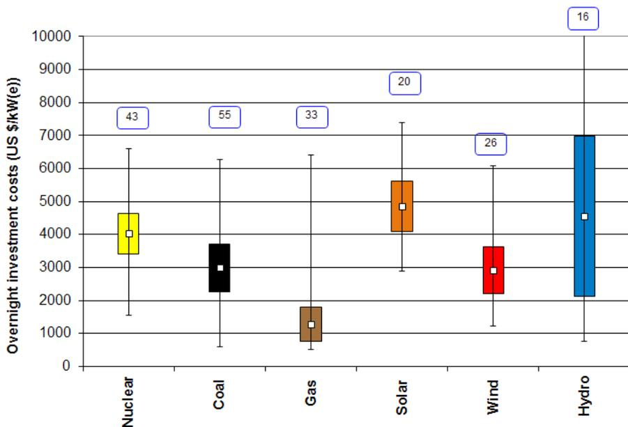
FIG. 22. Overnight investment cost estimates for the main electricity generation technologies. Data source: Ref. [77]. Note: This chart is based on data compiled from sources published between 2010 and 2013.
