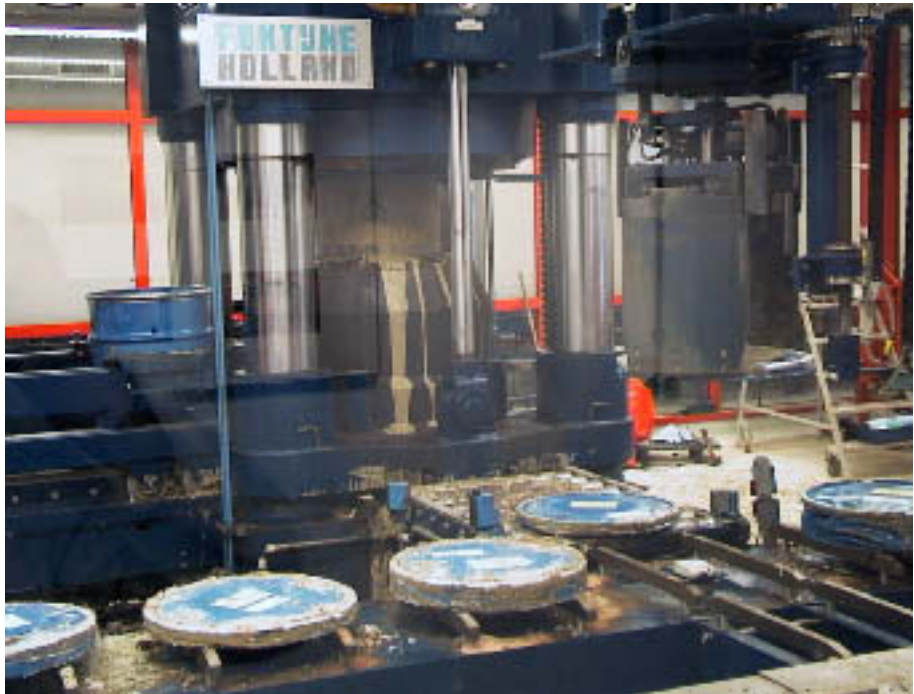
FIG. 3. The supercompactor at COVRA in the Netherlands.
