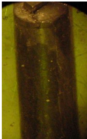
Fuel pin heated at 700°C
