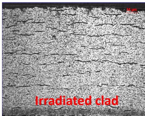
FIG. 6. Circumferential hydrides in the irradiated clad (irdd1).
