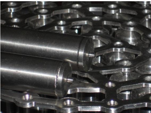
FIG. 6: present CARA fuel rod, end cap and end plate.
