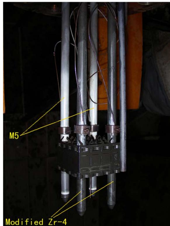
(a) Elements group after 3000h test in 4# water condition.
