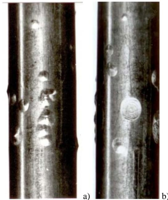
*FIG. 8. Nodular corrosion on CANDU fuel rod Zy-4 cladding tested 90 days in TRIGA reactor using irradiation capsule.*
