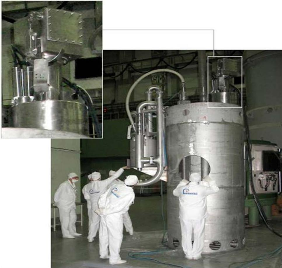
*FIG. 2. UP in standard housing, type 12. Workers of the plant and representatives of OKB “Gidropress” are examining the pump-filtering equipment. The frame in the figure highlights the cylindrical vessel of the plant, the loading chamber, hoses and insulated power cables. The pump-filtering facility and connecting flexible hoses are located on the housing of type 12 on the left.*
