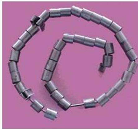
FIG. 3. Samples of tubes for weight gain measurement.
