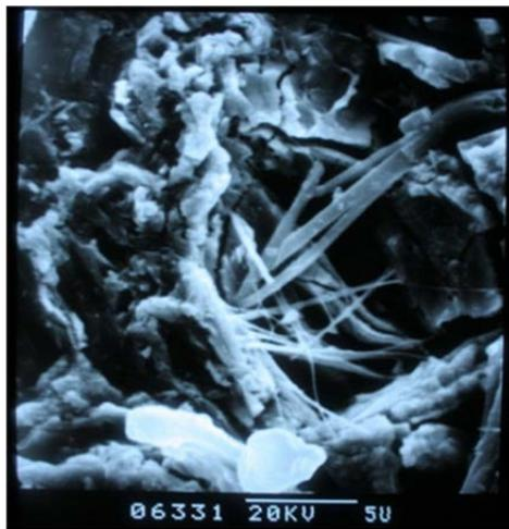
(c) Pores in the crud layer of M5 elements
