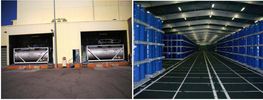
FIG. 1. Emptying of uranium nitrate from LR65 tank containers at TU5 (left) and interim storage in P35 (right).
