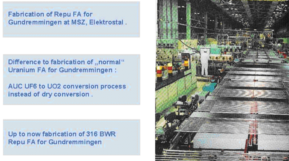
FIG. 1. Fabrication of ERU FA for the BWR Gundremmingen B.
