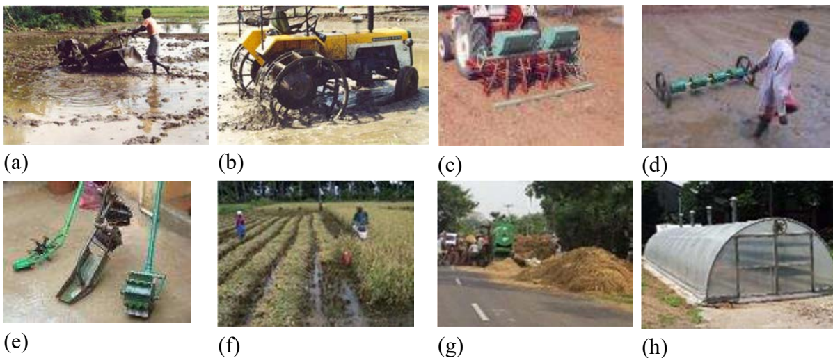
FIG. 3.31. Examples of appropriate mechanization: selected farm machines suitable for small holder farmers: (a) Power tiller; (b) Tractor with cage wheels; (c) Drill seeder cum fertiliser applicator; (d) Drum seeder; (e) Rotating hoe weeders; (f) Reaper harvester; (g) Mobile thresher; and (h) Plastic dome for drying rice grain (Photos by V. Balasubramanian).
