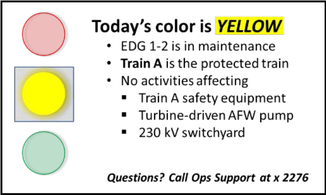
FIG. 35. Example for communicating basic plant risk configuration.
