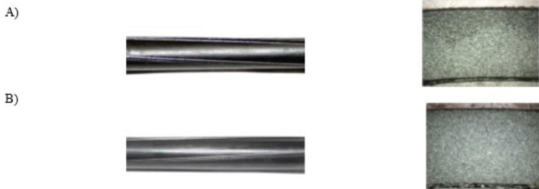
FIG. 2. Dependence of oxide film layer thickness at the surface of ferritic-martensitic steel from time of corrosion testing ( T=600^{\circ}\text{C} )
