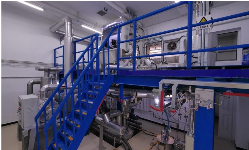
FIG. 3. The picture of the LBE dynamic corrosion test loop
