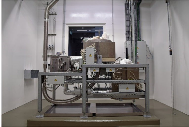
FIG.2. View of the LILLA experimental facility for mechanical testing in liquid lead
