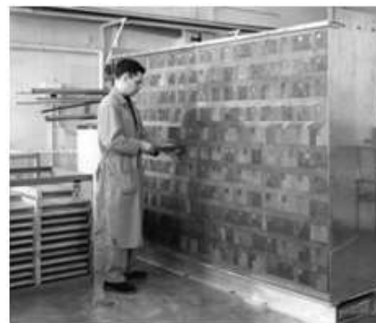
FIG. VI-4. Graphite pile configured for neutron moderation measurements.
