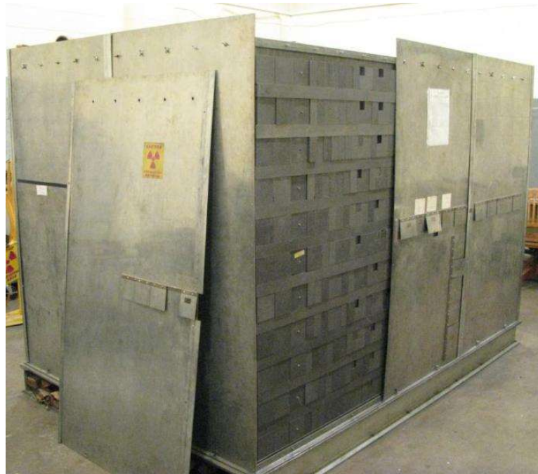
FIG. VI-1. Penn State Graphite Subcritical Reactor (cadmium cover partially removed).
