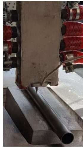
FIG. 46. Device used for Blister formation (courtesy of CNEA).
