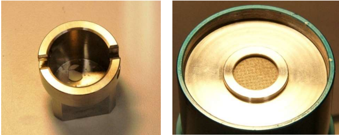
FIG. 57. Big fragments are collected in the container placed at the bottom of the funnel (left), fine fragments/aerosol particles are collected on the metallic filter (right) (courtesy of JRC-Karlsruhe).
