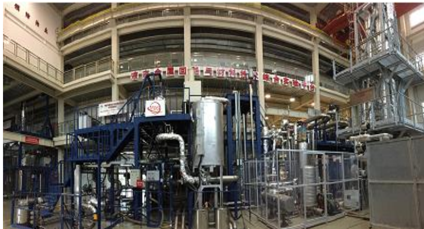
FIG. 1. Multi-functional lead-bismuth loop KYLIN-II [16]
