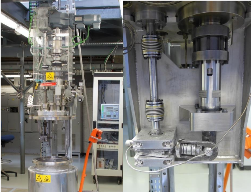
FIG. 7. The RHAPTER facility: the installed facility and a close-up of a bearing testing module
