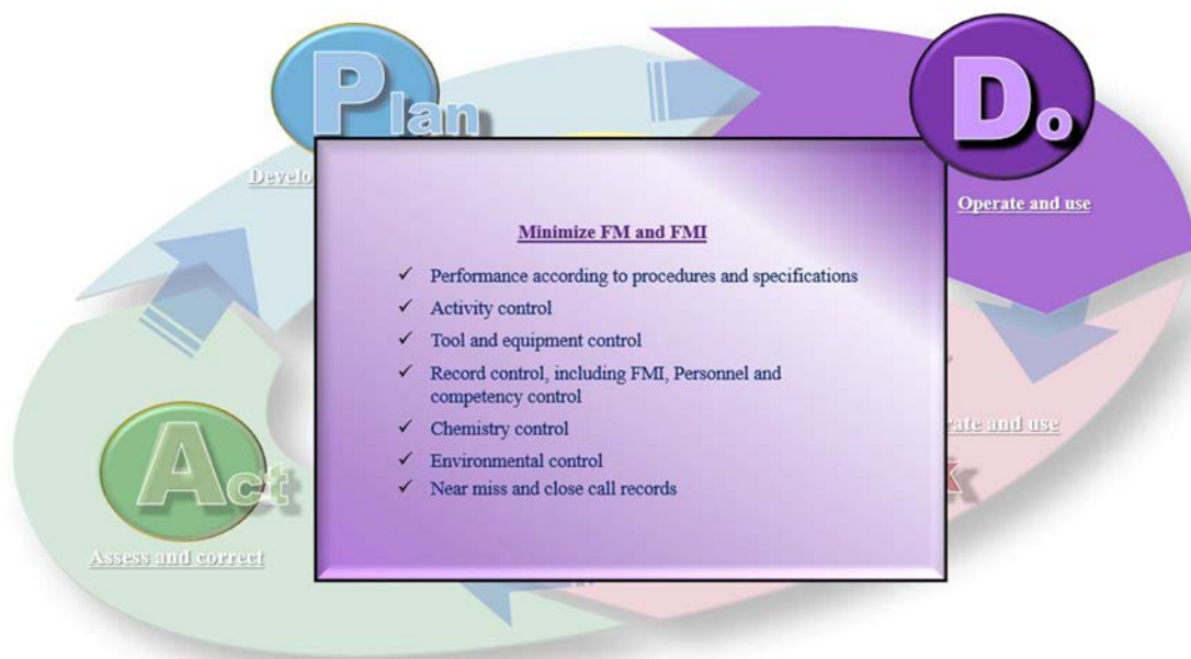
FIG. 11. Application, implementation and performance of foreign material management: 'Do'. FMI —foreign material intrusion, FM —foreign material.
