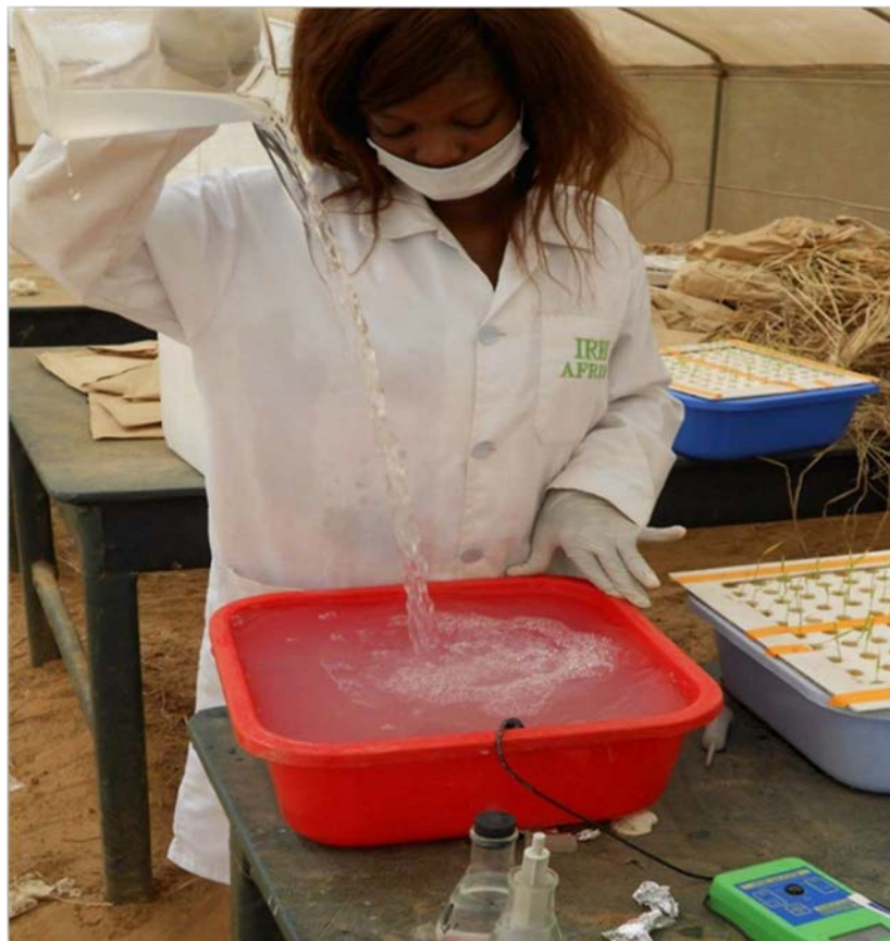
FIG. 4. Chemical preparation of Yoshida nutrient solution and measurement of pH and EC of the experimental set up.
