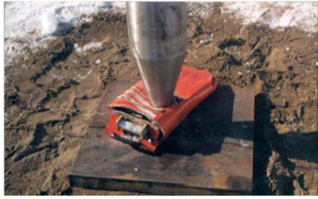
FIG. 26. View of probe embedded in FDR. Reproduced courtesy of Institute of Nuclear Materials Management [4]
