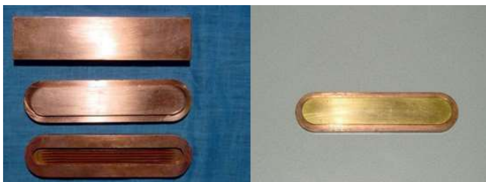
FIG. 19. (Left) The copper target body surfaces (unfinished target (up), electroplating surface (middle) and water-cooled surface (below) and (right) gold-plated target used for zinc electroplating (courtesy of A. Jalilian, IAEA, Austria).
