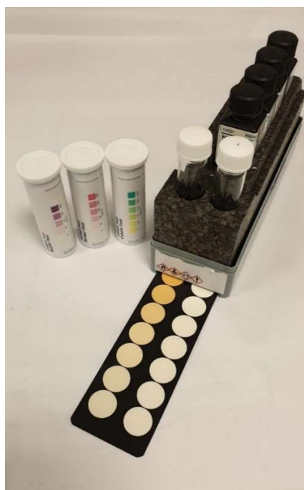
FIG. 21. Commercially available semi-quantitative metal detection test strips and colour card comparator kit (courtesy of K. Gagnon, GE healthcare, Sweden).
