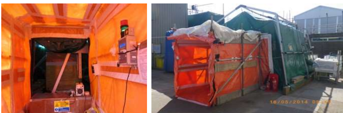
FIG. 6. Containment tent, similar to those used by the emergency services in response to chemical and radiological incidents for personnel treatment and decontamination (courtesy of Bradwell, United Kingdom).
