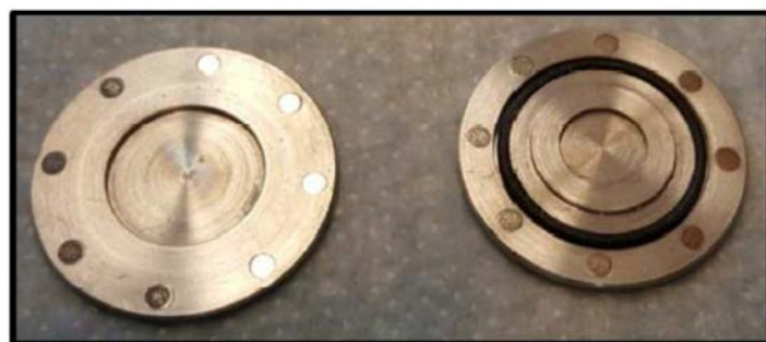
FIG. 22. Powder titanium oxide target folder (Courtesy of Ms. Lapi, University of Alabama, USA).
