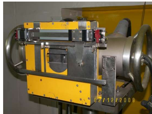
FIG. 39 (A&B). (A) Digitally controlled fast X ray shutter mechanism (B) Shutter assembly mounted on the X ray tube head on top of the beam collimator
