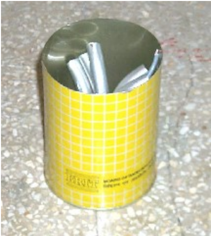
FIG.31. Photograph of the specimen – a commercial thin metallic container [100mm(H)x100mm (OD)] housing a section of welded aluminium curved tubes (12 nos.). The container was partially filled with water.
