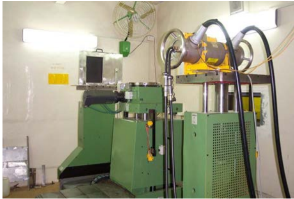
FIG. 37. Photographic view of the X ray based Direct Digital Radiography and Volume Tomography System housed inside a shielded enclosure
