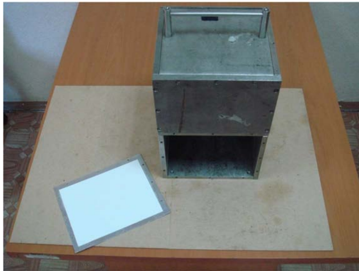
FIG.34. A typical assembled fluoroscope and fluorescent screen developed by Germany's Federal Institute for Materials Research and Testing (BAM) (Image courtesy: IAEA Radiation Technology Report No. 2 (2013) published by International Atomic Energy Agency, Vienna)
