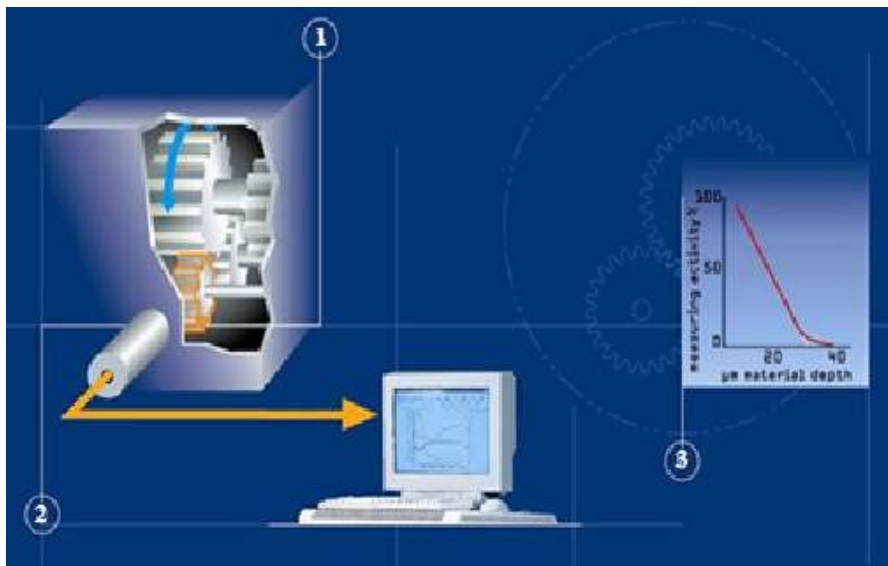
FIG. 19. Schematics of the direct measurement setup; 1. Activated part 2. Detector 3. Calibration curve (activity versus depth in the material) [38].
