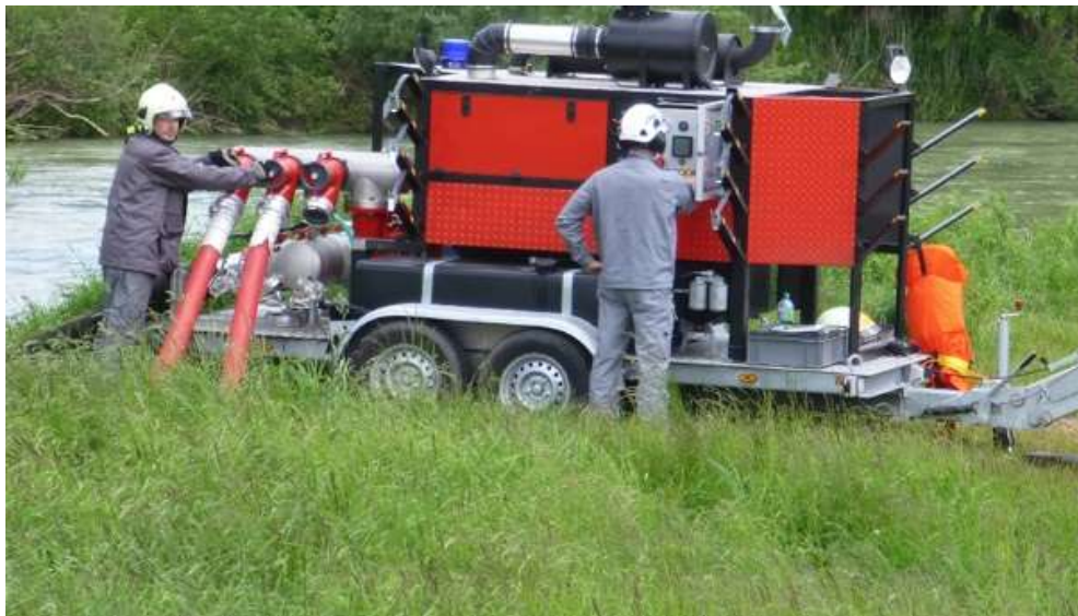
FIG. I-21-6. Fire water pump, one necessary, three stationed at the plant.
