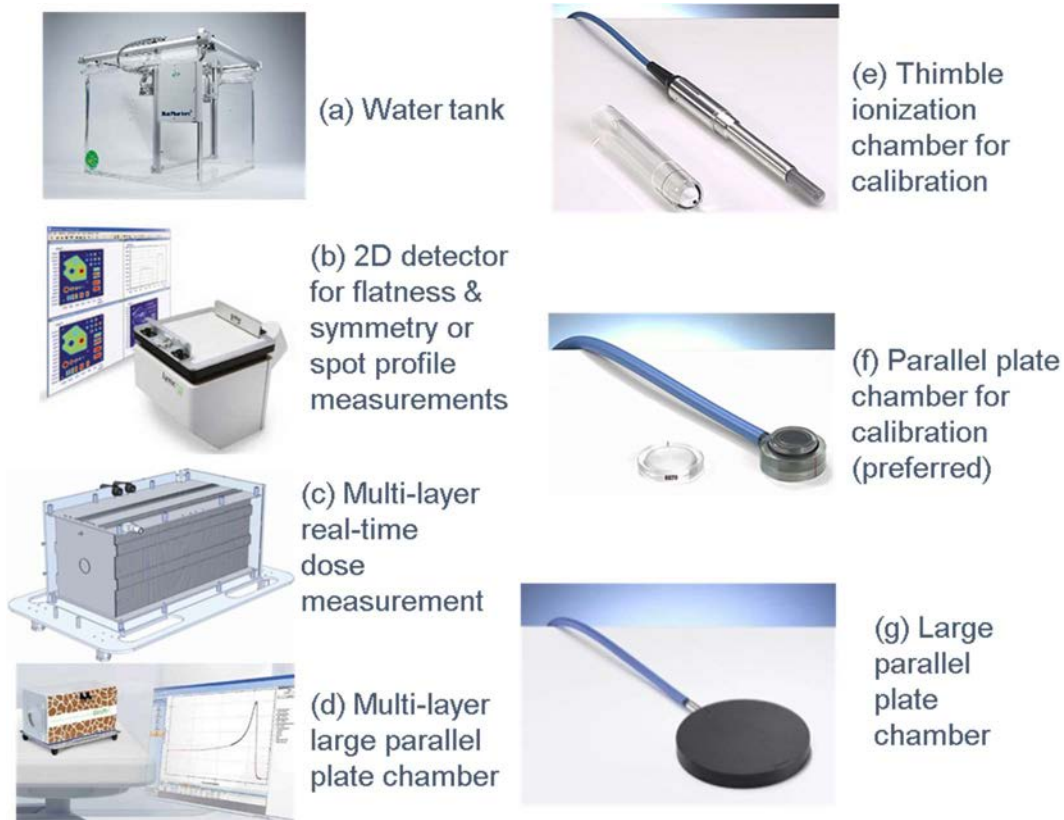
FIG. 27: Examples of equipment for ion beam dosimetry measurements: (a) water tank; (b) 2-D scintillation detector for high resolution measurement; (c) multi-layer ion chamber array for real-time central-axis depth dose measurement; (d) multi-layer large parallel plate chamber array for real-time integrated pencil beam dose measurement; (e) thimble ion chamber for dose calibration; (f) parallel plate chamber for dose calibration; (g) large parallel plate chamber for pencil beam scanning commissioning.
