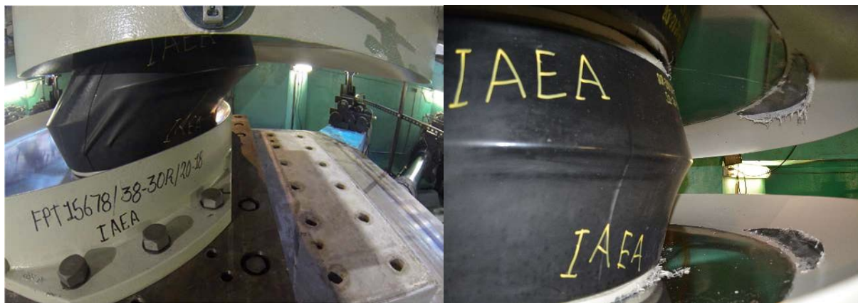
FIG. 119. Behaviour of TPFB when hardening stage initiates. (a) Large displacement of the bearing into the hardening stage. (b) Yielding mechanism and damage of rim and slider edge after the run.
