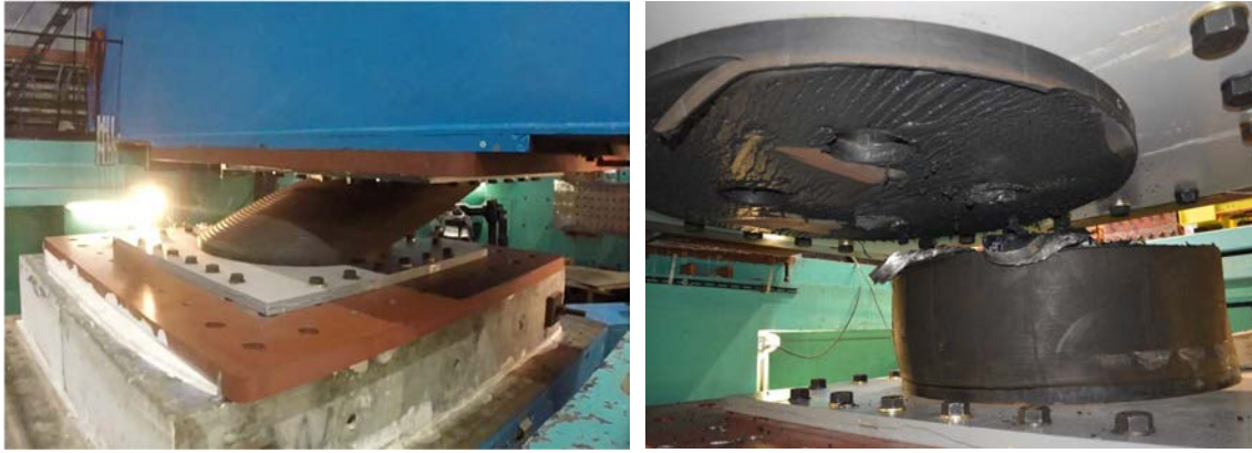
FIG. 101. Failure mechanism of LRB specimen (UET2). (a) Large horizontal shear strain before failure. (b) Failure observed between rubber and steel shim and extreme deformation of lead cores.
